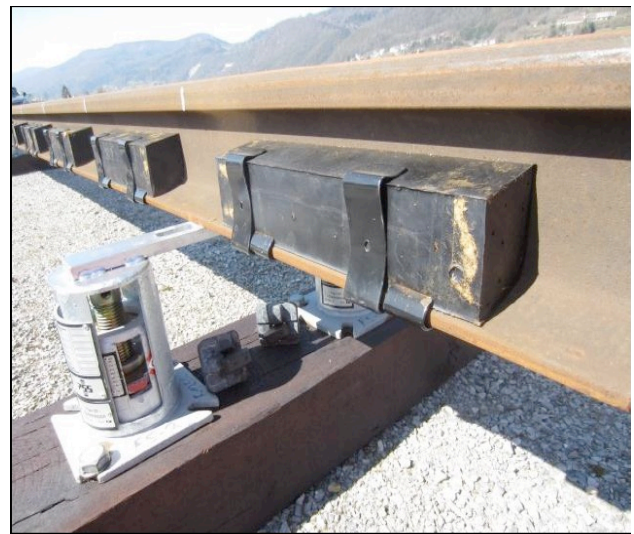
Fig. 13. TATA Steel damping rail [16].
