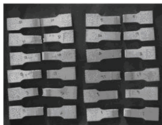
Figure 5. Tensile specimen after fracture
