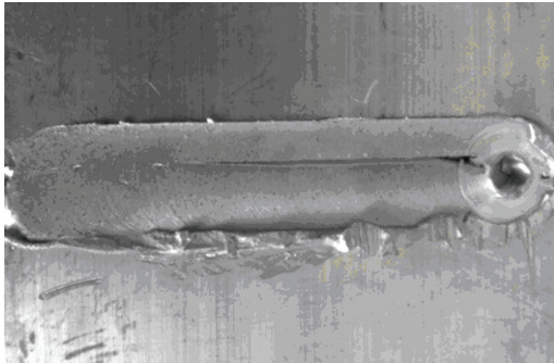
Figure 3. Typical FS welded plate having tunneling defect in welded area
