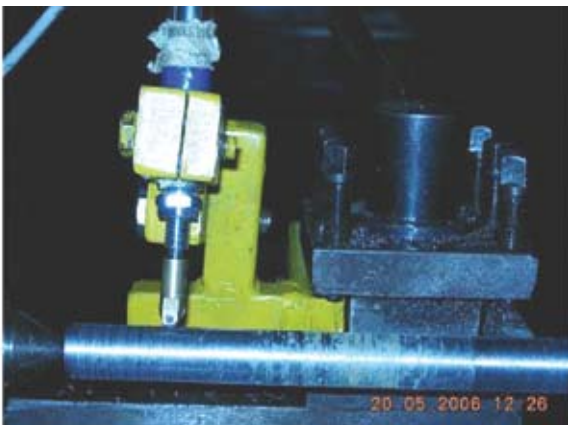
Figure 1. LVDT Set up
