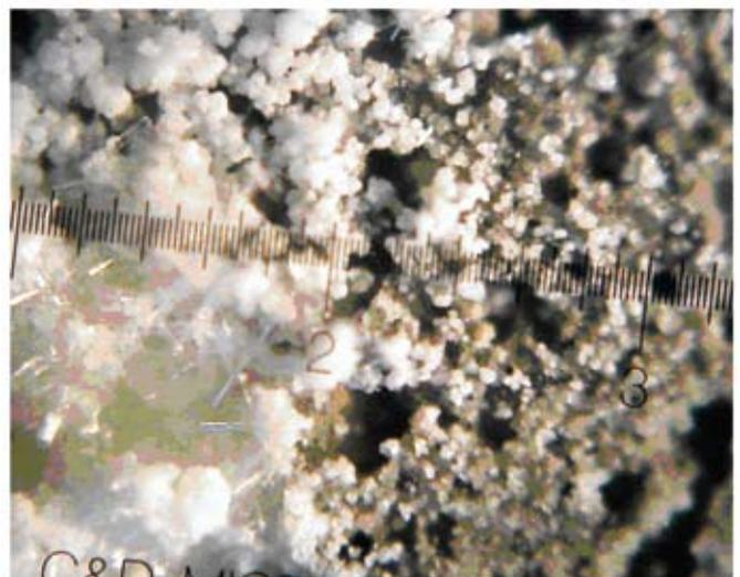
**Figure 1.** Needle like structures observed on the surface of specimen after 6 weeks exposure.
