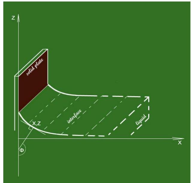
**Figure 5.** An interface meeting a plane wall ( $x=0$  plane) with some contact angle. The meridian angle  $\Phi$  is shown.
