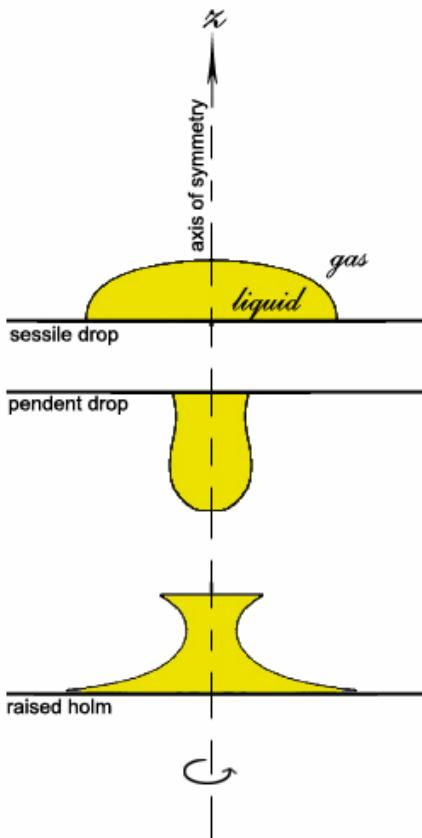
**Figure 4.** Meridians for axisymmetric fluid bodies in a gravitational field.
