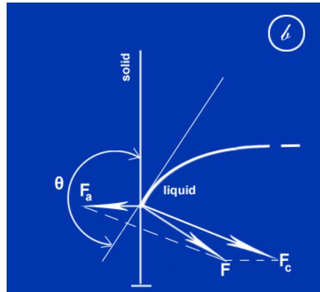
Figure 1. Cohesion and adhesion forces.
