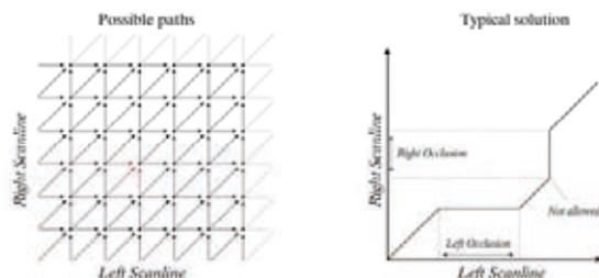
**Fig. 2** Minimizing path (on the right) is determined by calculating recursively a cost function. Each point in the cost function (on the left) is derived from the three previous values, as shown by the arrows. Disparities are tallied in a next stage, by backtracking the path of minimum cost.
