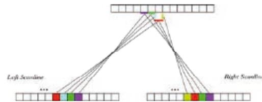
**Fig. 1** The monotonic ordering constraint in stereo-vision. Finding the correspondence between two conjugate points in a stereo-pair means that all other correspondences lie to the right of the two points in both left and right images.
