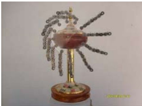
Fig. 6. Picture of our perpetual motion machine, which is a version of Arabian Perpetuum Mobile.
