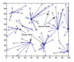
Fig. 1. Snapshot of cluster foundation in LEACH for 100 nodes.
