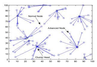
Fig. 3. Snapshot of cluster foundation in SEP for 100 nodes.
