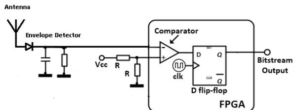
Fig. 5 Wireless receiver and demodulator implementation.
