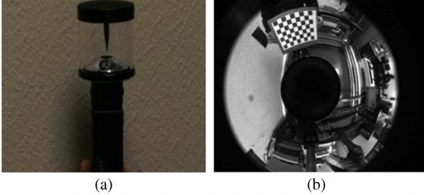
Fig. 1 Implementation of omnidirectional video cameras by using paraboloidal mirrors. [4]
