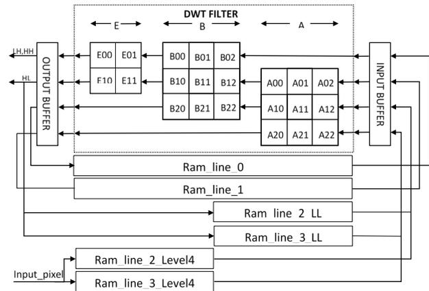
Fig. 2 SCLA algorithm block diagram of DWT core with the memories used.
