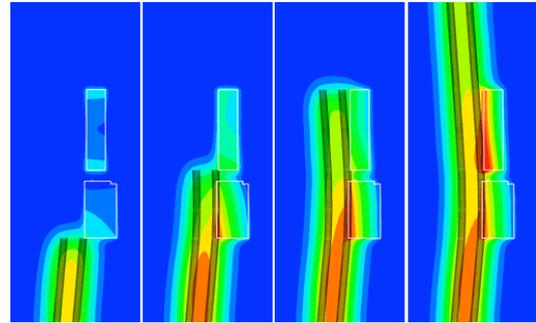
Fig.9. Cloud chart of buildings and ground deformation after shield construction
