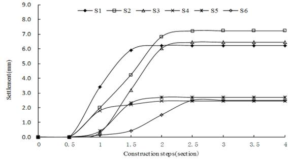
Fig.11. Chart of the settlement in monitoring points
