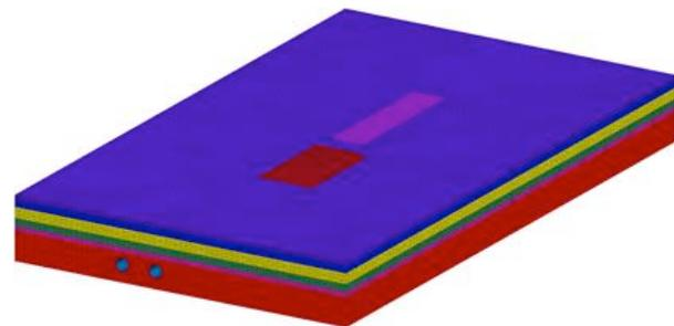
Fig.4. Position relationship between the running tunnel and the existing building
