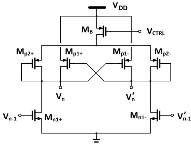
Fig. 4. Delay element with controllable current source
