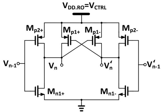
Fig. 7. Proposed delay element with CMOS inverters
