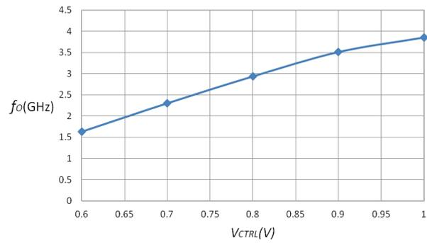
**Fig. 8.** Simulated oscillation frequency versus  $V_{CTRL}$
