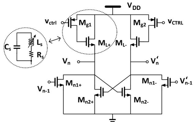
Fig. 6. Delay element with active inductors
