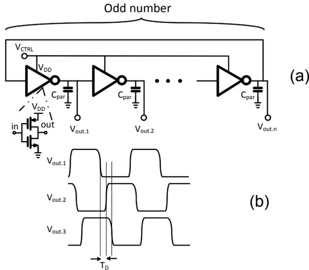
Fig. 1. (a) RO basic single ended topology with CMOS inverter based delay element and (b) output waveforms
