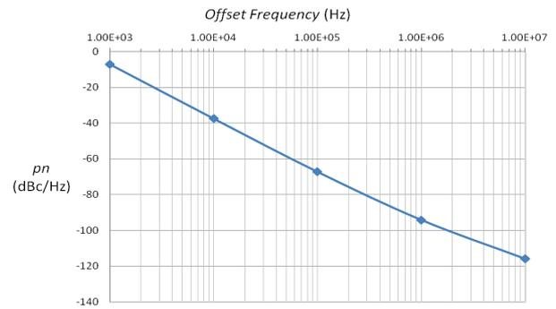
**Fig. 9.** Phase noise versus offset frequency
