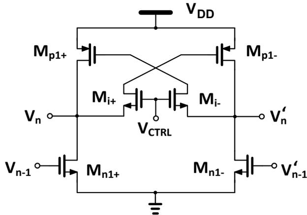
Fig. 3. Delay element with controllable latch
