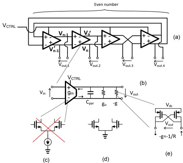
Fig. 2. (a) Differential RO (b) block diagram of delay element (c) fully differential gm stage (d) pseudo-differential gm stage and (e) basic structure of active differential negative conductance -g.
