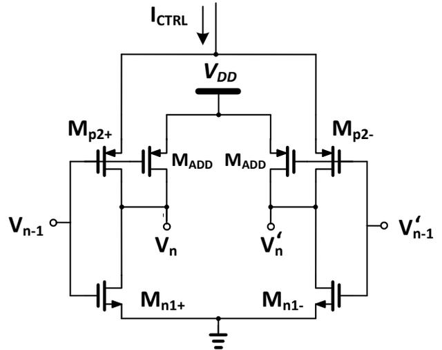
Fig. 5. Delay element with controllable current-starved inverters
