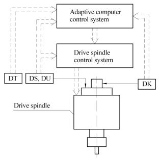
Fig. 3. Principal movement module structure.
