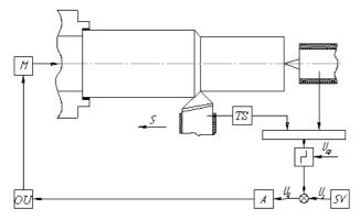
Fig. 2. Flow chart of a subsystem controlling the speed depending on the cutting temperature.
