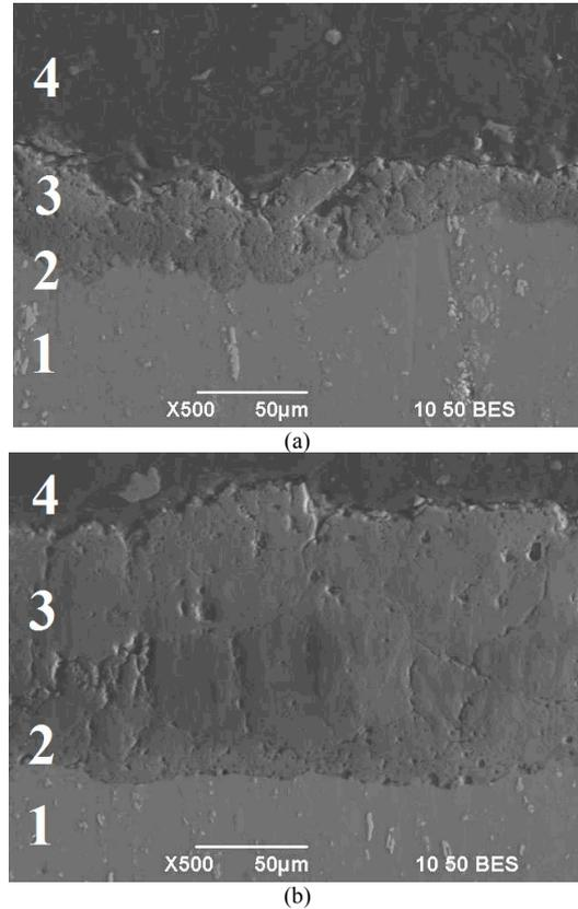
**Fig. 2.** Interface of AK12D alloy and MAO-layer: a) sample №1, b) sample №2; 1 – metal; 2 – transition layer; 3 – base layer; 4 – epoxide resin
