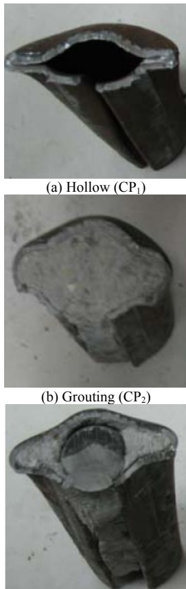
(c) Inserting steel bar (CP 3 ) Fig. 3. Shear fracture photos of bolts with seam
