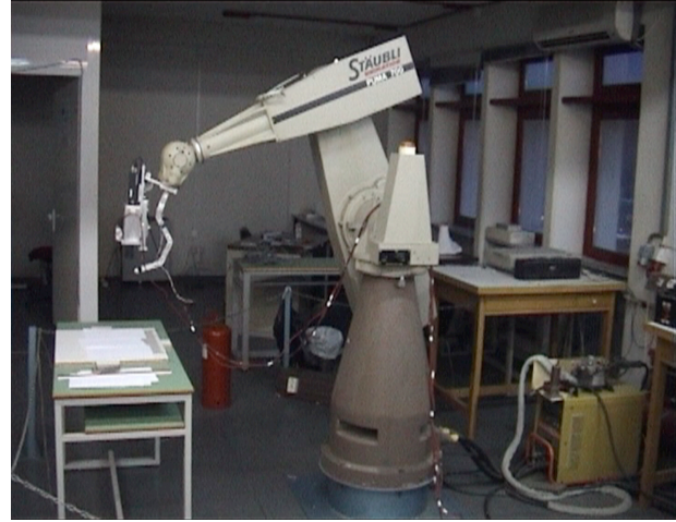
Photo 4. PUMA 761 performing a task based on PSVS.
