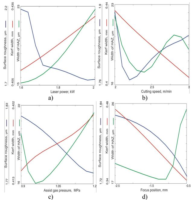
**Figure 1** Effect of laser cutting parameters on cut quality characteristics: a) effect of laser power, b) effect of cutting speed, c) effect of assist gas pressure, d) effect of focus position.
