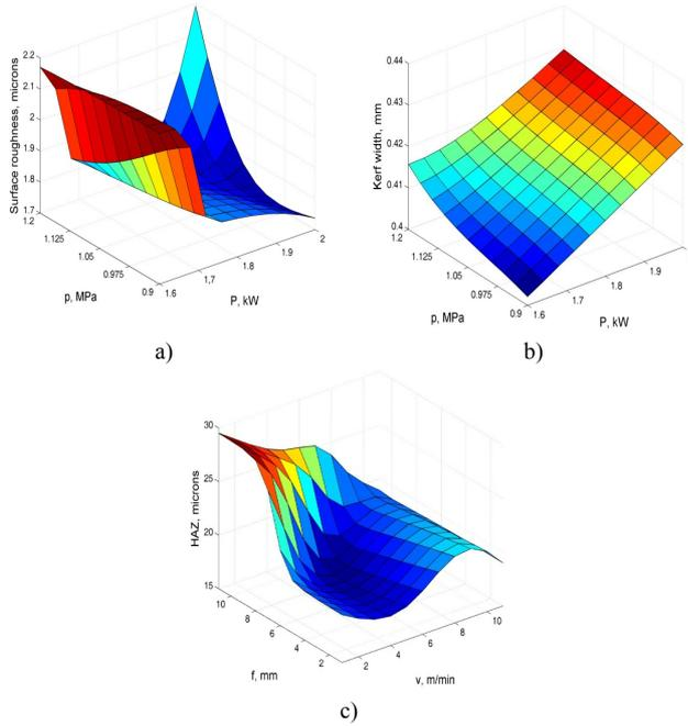
**Figure 2** Some interaction effect on the cut quality characteristics: a) interaction effect of laser power and assist gas pressure on surface roughness, b) interaction effect of laser power and assist gas pressure on kerf width, c) interaction effect of cutting speed and focus position on HAZ
