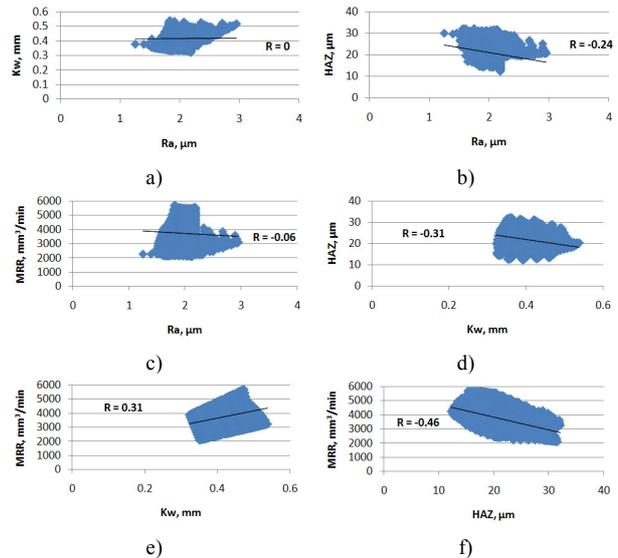
Figure 7 Trade-off operating diagrams for performance characteristics
