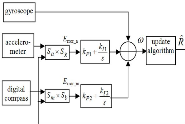
Fig. 10 The proposed algorithm structure of azimuth by complementary filter
