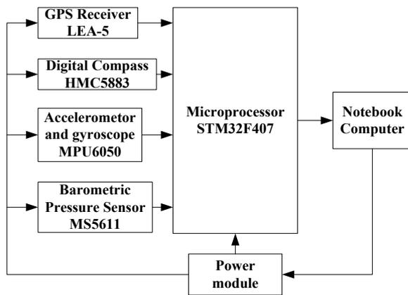
Fig. 1 The hardware system diagram of the proposed PDR system
