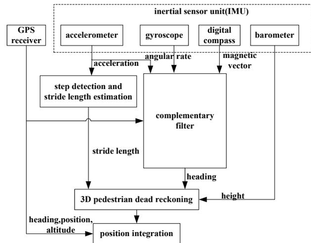
Fig. 2 The proposed algorithm structure
