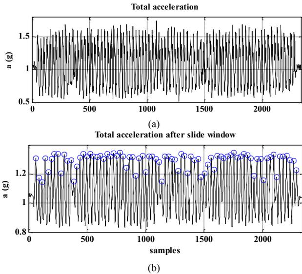
Fig. 9 step detection (a) total acceleration signal before filtering (b) after filtering
