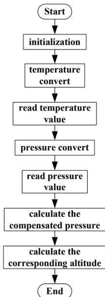
Fig. 7 The read process of MS5611
