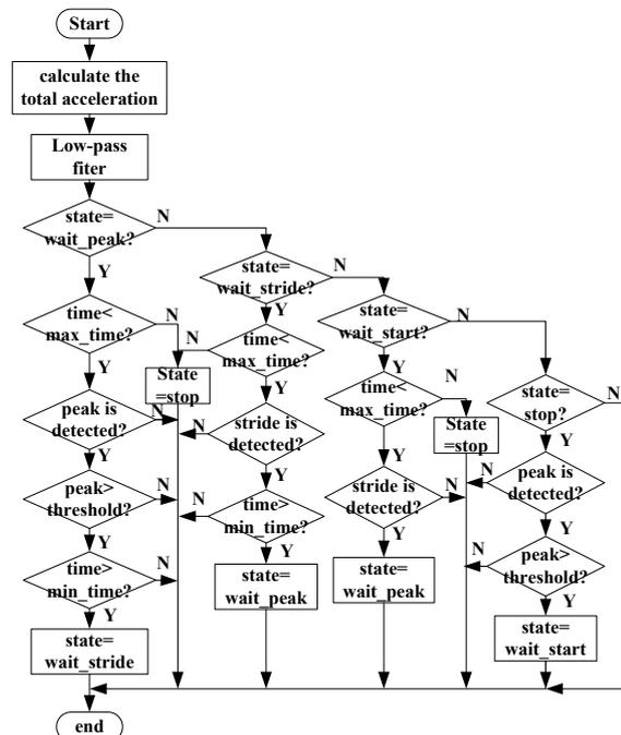
Fig. 8 The soft process of the step occurrence detection
