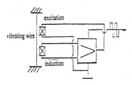
Fig.2. Operating Principle of Vibrating-wire
