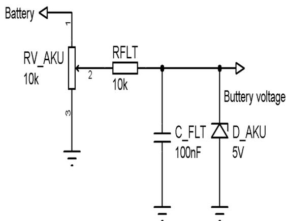
Fig. 9. Battery voltage measuring circuit
