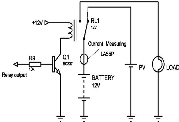
Fig. 4. Load and battery switching circuit
