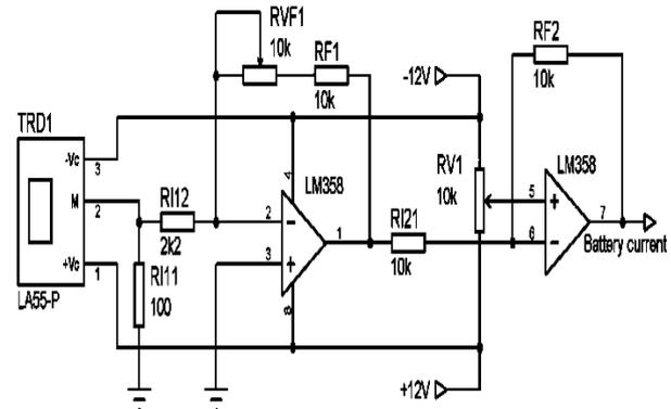
Fig. 7. Current to voltage converter circuit
