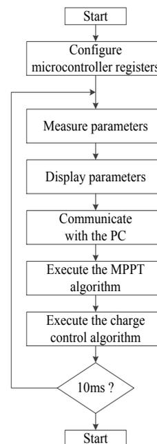
Fig. 11. Flowchart of microcontroller program
