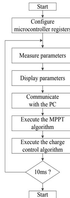
Fig. 11. Flowchart of microcontroller program
