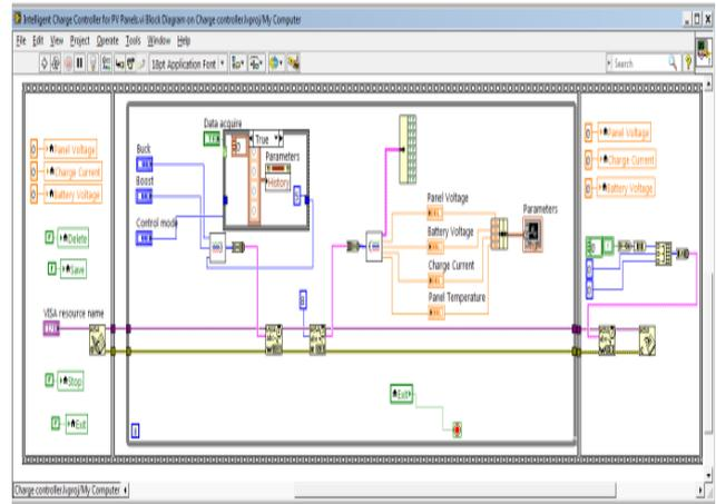
Fig. 13. Block diagram of VI
