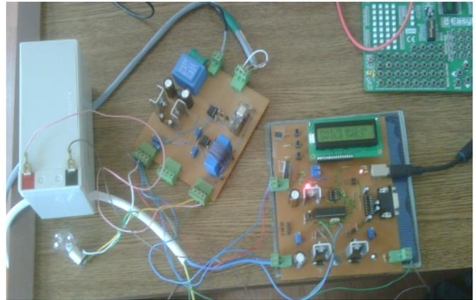
Fig. 10. The circuit of charge controller for PV panel
