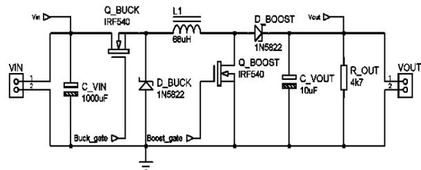
Fig. 2. The schema of buck-boost controller
