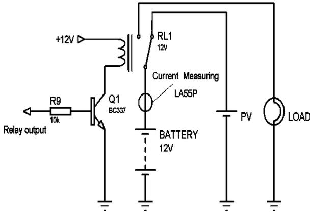
Fig. 4. Load and battery switching circuit
