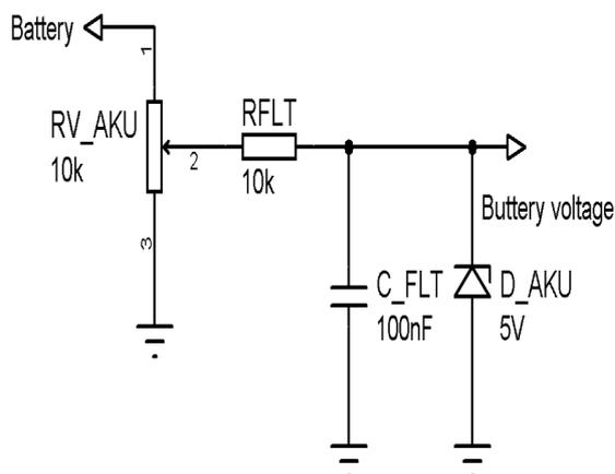
Fig. 9. Battery voltage measuring circuit
