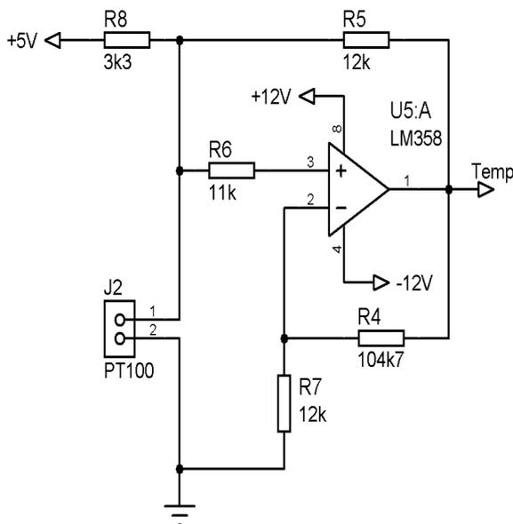
Fig. 5. The schema of PT100 amplification circuit
