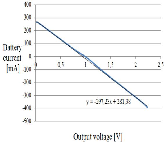
Fig. 8. Relationship between battery current and output voltage
