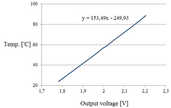
Fig. 6. Relationship between temperature and output voltage
