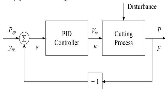
Fig. 2. Control loop with PID controller
