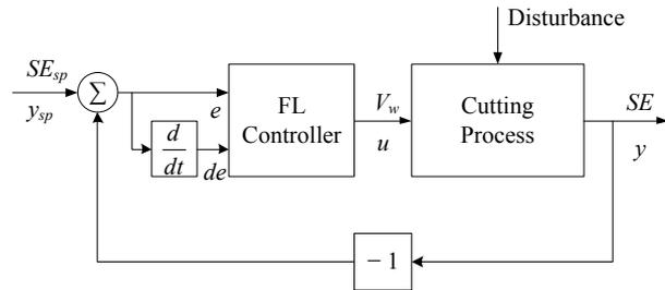
Fig. 3. Control loop with FL controller
