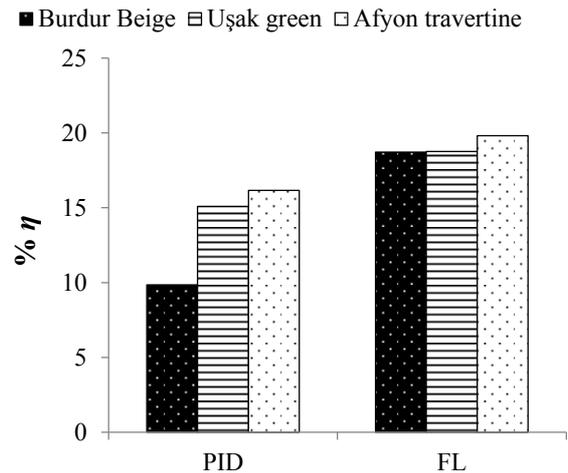
Fig. 13. Mean of energy saving values for control methods
