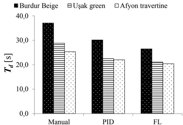
**Fig. 11.** Mean of durations for control methods
