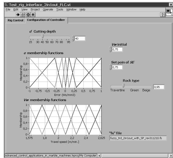
Fig. 6. Controller configuration tab
