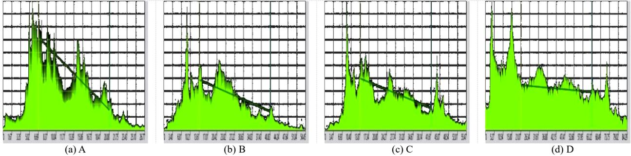
Fig. 11. Surface height measurement maps of the specimen under different cleaning conditions (700×)
