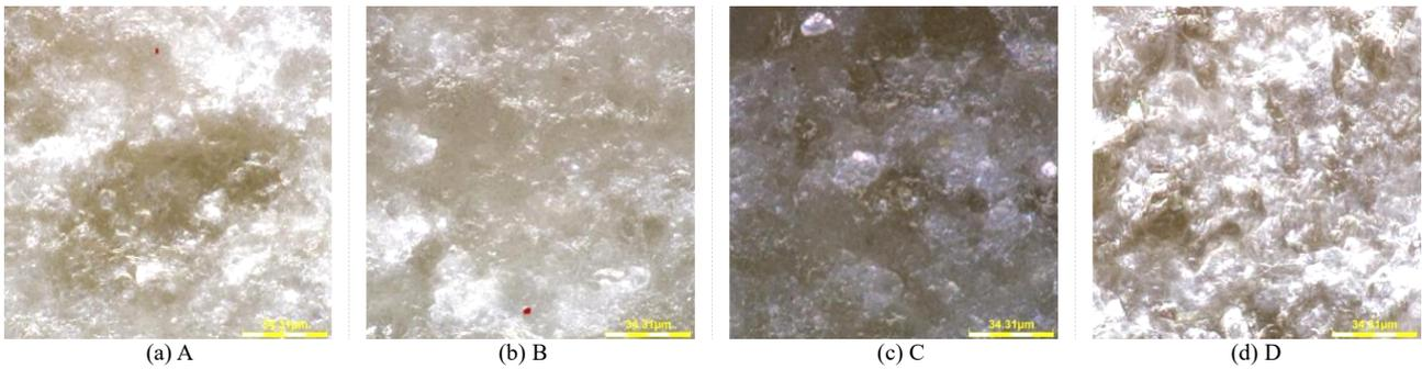
Fig. 10. Microscopic images of the surface damage morphology of the specimen after treatment under different cleaning conditions (2000×)
