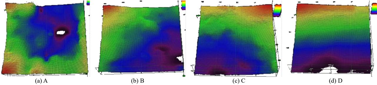
Fig. 9. 3D high-depth-of-field images of surface damage of test blocks under different cleaning conditions (700×)
