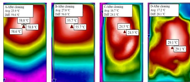
Fig. 4. Infrared thermal imaging of test block after steam cleaning
