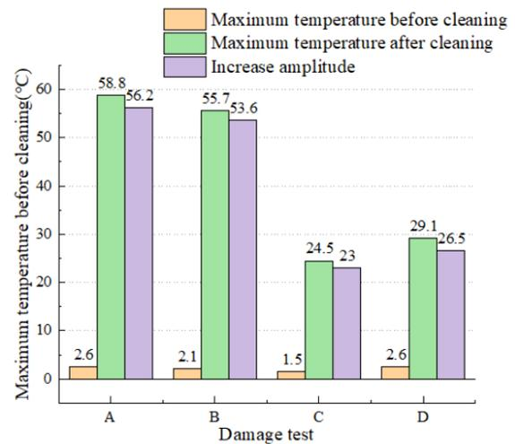
Fig. 6. Temperature variation on test block surface before and after cleaning
