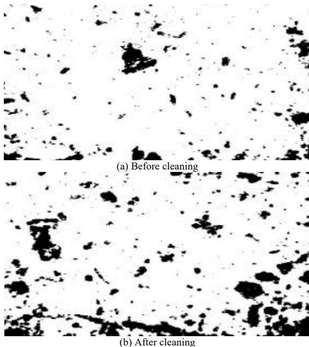
Fig. 7. Binary image of test block before and after steam cleaning
