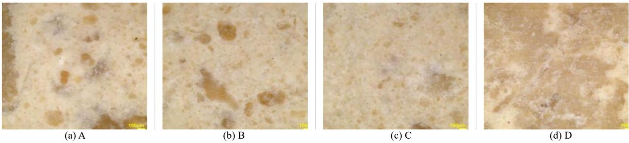
Fig. 8. High-definition digital photos of surface damage of test blocks under different cleaning conditions (700×)
