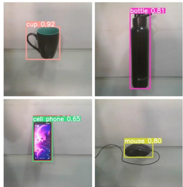
Fig. 8. Model predicts object name, displays bounding boxes on images.
