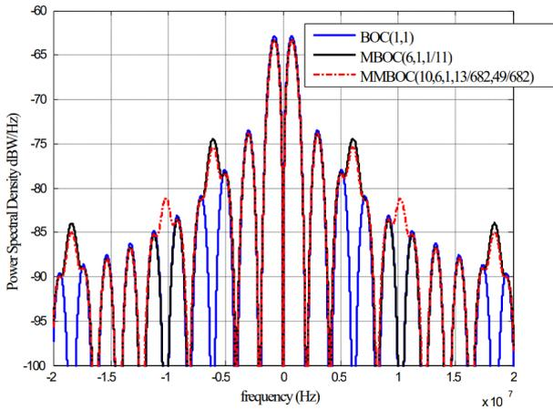
Fig. 2. Normalized PSDs of BOC, MBOC and MMBOC
