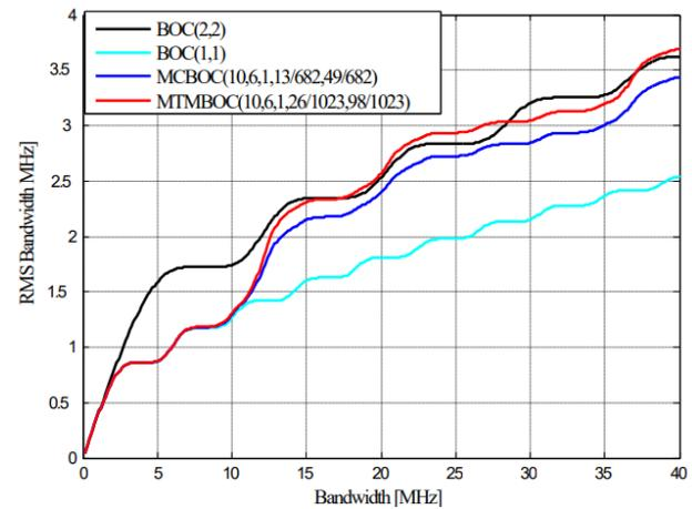
**Fig. 16.** RMSB of BOC(1, 1), BOC(2, 2), MCBOC(10, 6, 1, 13/682, 49/682) and MTMBOC(10, 6, 1, 26/1023, 98/1023).
