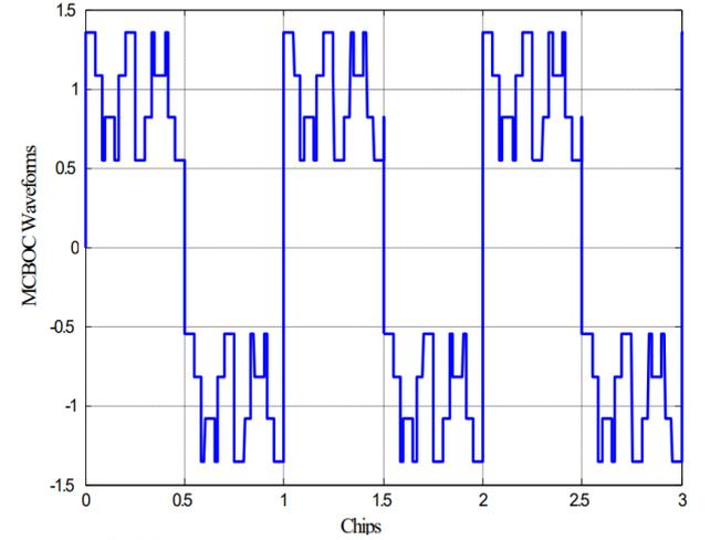
Fig. 4. MCBOC modulated signal
