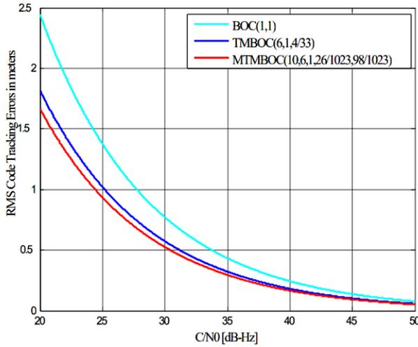
**Fig. 12.** RMS Code Tracking Errors of BOC(1, 1), TMBOC(6, 1, 4/33) and MTMBOC(10, 6, 1, 26/1023, 98/1023) with 24 MHz front-end bandwidth
