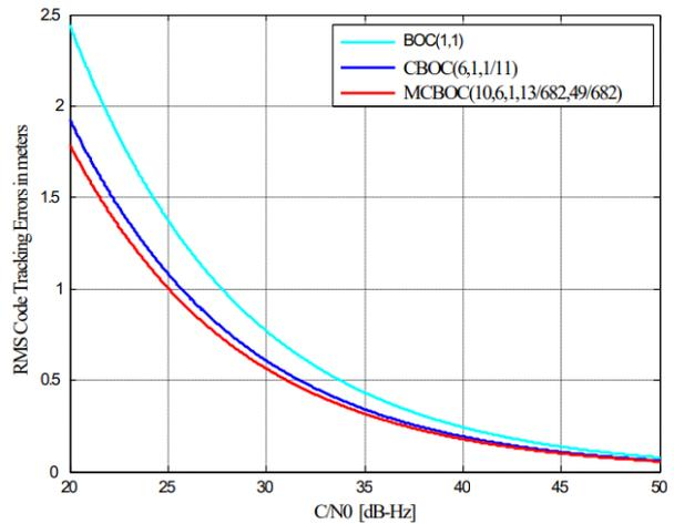
Fig. 11. RMS Code Tracking Errors of BOC(1, 1), CBOC(6, 1, 1/11) and MCBOC(10, 6, 1, 13/682, 49/682) with 24 MHz front-end bandwidth.
