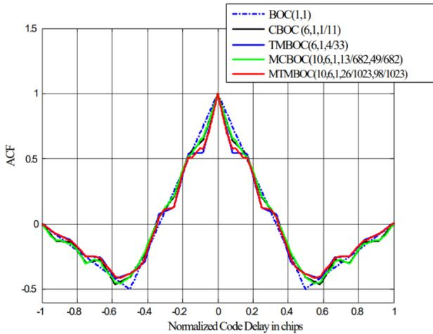
Fig. 10. Normalized ACFs of BOC(1, 1), CBOC(6, 1, 1/11), TMBOC(6, 1, 4/33), MCBOC(10, 6, 1, 13/682, 49/682) and MTMBOC(10, 6, 1, 26/1023, 98/1023).
