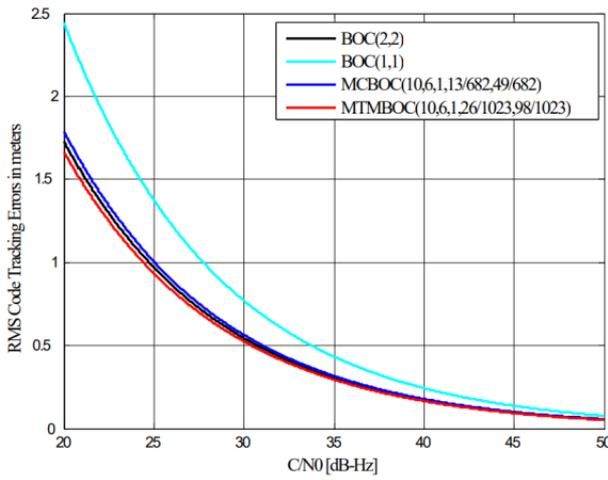
**Fig. 13.** RMS Code Tracking Errors of BOC(1, 1), BOC(2, 2), MCBOC(10, 6, 1, 13/682, 49/682) and MTMBOC(10, 6, 1, 26/1023, 98/1023) with 24 MHz front-end bandwidth.
