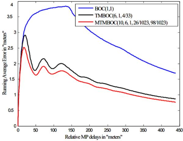
Fig. 19. RAEs of BOC(1, 1), TMBOC(6, 1, 4/33) and MTMBOC(10, 6, 1, 26/1023, 98/1023).
