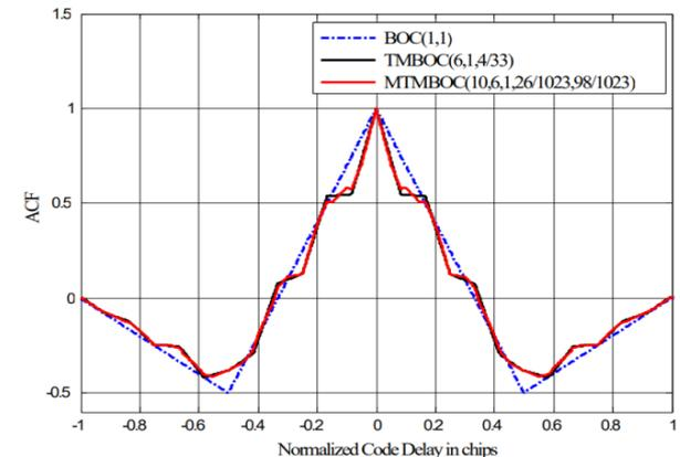
**Fig. 7.** Normalized ACFs of BOC(1, 1), TBOC(6, 1, 4/33), and MTMBOC(10, 6, 1, 26/1023, 98/1023).
