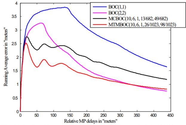
Fig. 21. RAEs of BOC(1, 1), BOC(2, 2), MCBOC(10, 6, 1, 13/682, 49/682) and MTMBOC(10, 6, 1, 26/1023, 98/1023)
