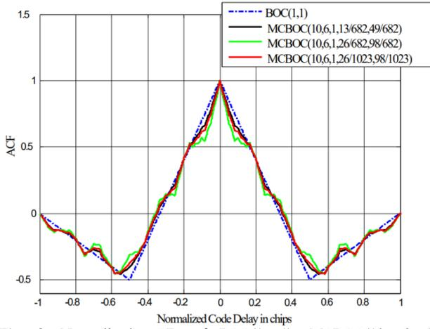
Fig. 8. Normalized ACFs of BOC(1, 1), MCBOC(10, 6, 1, 13/682, 49/682), MCBOC(10, 6, 1, 26/682, 98/682), and MCBOC(10, 6, 1, 26/1023, 98/1023).
