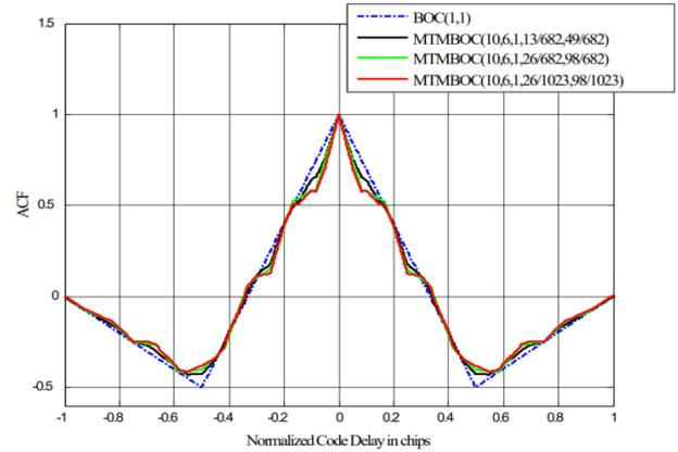
**Fig. 6.** Normalized ACFs of BOC(1, 1), MTMBOC(10, 6, 1, 13/682, 49/682), MTMBOC(10, 6, 1, 26/682, 98/682) and MTMBOC(10, 6, 1, 26/1023, 98/1023)
