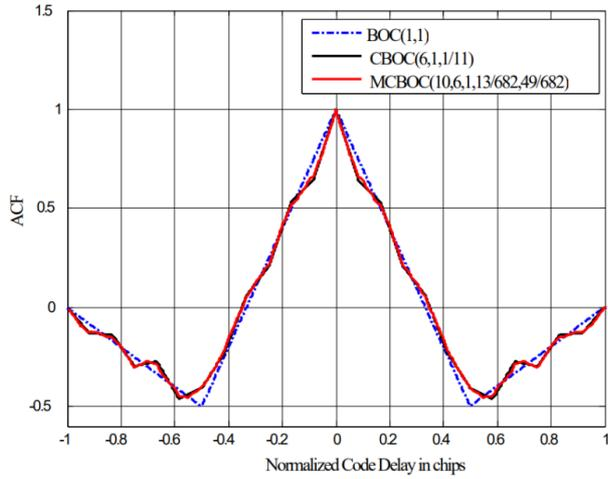
Fig. 9. Normalized ACFs of BOC(1, 1), CBOC(6, 1, 1/11), and MCBOC(10, 6, 1, 13/682, 49/682)
