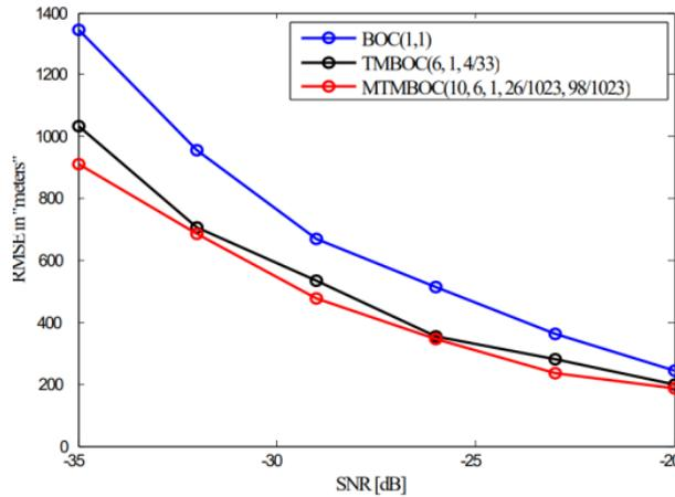
Fig. 22. RMSEs of BOC(1, 1), TMBOC(6, 1, 4/33) and MTMBOC(10, 6, 1, 26/1023, 98/1023).
