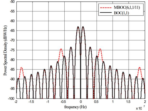
Fig. 1. Normalized PSDs of MBOC and BOC
