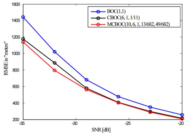
Fig. 23. RMSEs of BOC(1, 1), CBOC(6, 1, 1/11) and MCBOC(10, 6, 1, 13/682, 49/682).
