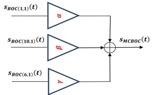
Fig. 5. Block diagram illustrating the generation of the MCBOC subcarrier
