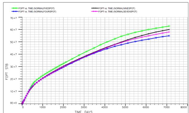
Fig. 15. Field Oil Production Total for Normal Flood Patterns
