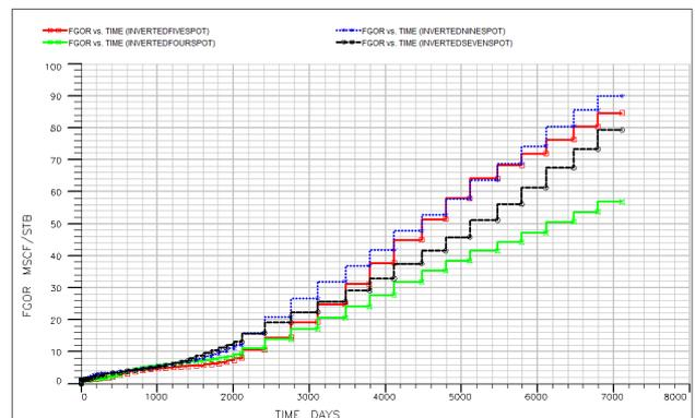
Fig. 14. Field Gas Oil Ratio for Inverted Flood Patterns
