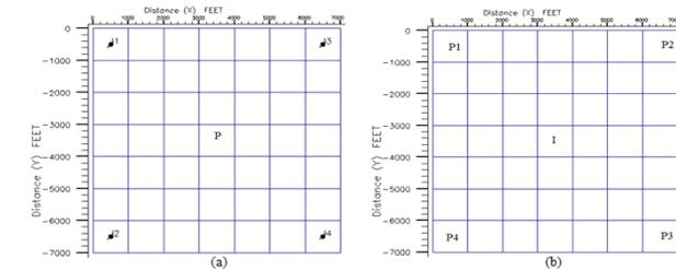
Fig. 7. (a) Normal Five Spot and (b) Inverted Five Spot
