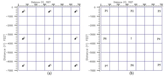
Fig. 9. (a) Normal Nine Spot and (b) Inverted Nine Spot
