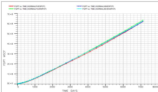
Fig. 17. Field Gas Production Total for Normal Flood Patterns
