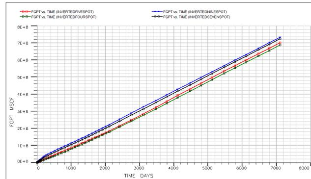
Fig. 18. Field Gas Production Total for Inverted Flood Patterns
