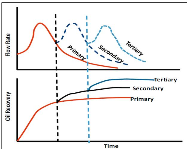
Fig. 2. Variation of flow rate and oil recovery for each oil recovery process [2]
