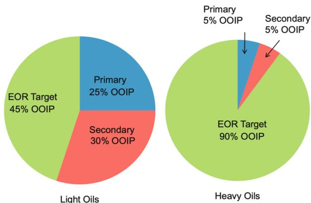
Fig. 1 Oil Recovery Target for Oil Recovery Processes for different crudes [2]
