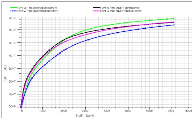
Fig. 16. Field Oil Production Total for Inverted Flood Patterns
