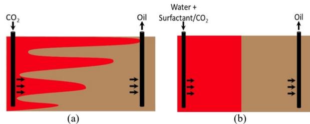
Fig. 4. Comparison of the sweep of oil between (a) gas flooding and (b) foam flooding [10]
