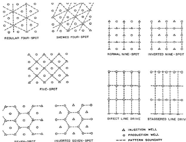
Fig. 5. Flooding patterns [17]
