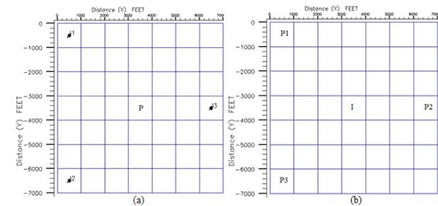
Fig. 6. (a) Normal Four Spot and (b) Inverted Four Spot
