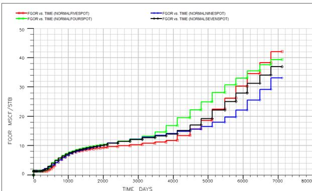
Fig. 13. Field Gas Oil Ratio for Normal Flood Patterns
