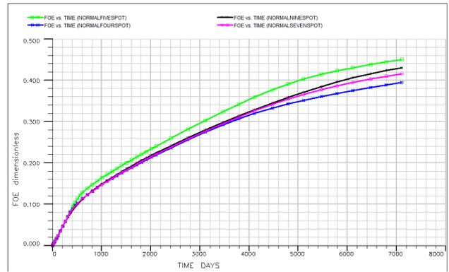
Fig. 11. Field Oil Efficiency for Normal Flood Patterns
