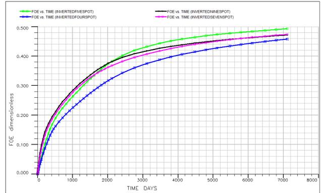
Fig. 12. Field Oil Efficiency for Inverted Flood Patterns
