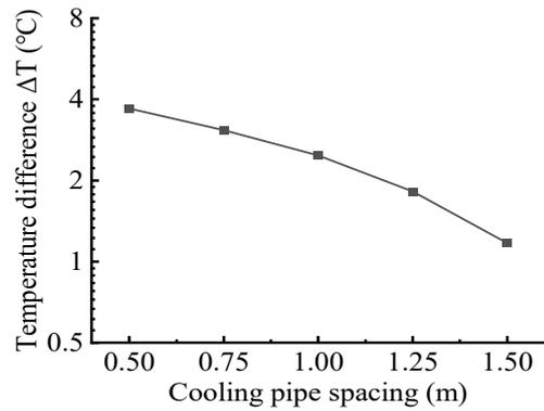
**Fig. 19.** Maximum temperature difference curve without and with cooling pipe
