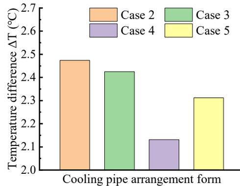
**Fig. 16.** Comparison diagram for the maximum transient temperature difference between caps with and without a cooling pipe
