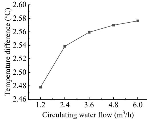
Fig. 23. Maximum temperature difference curve between the conditions without cooling pipe and with different water flows
