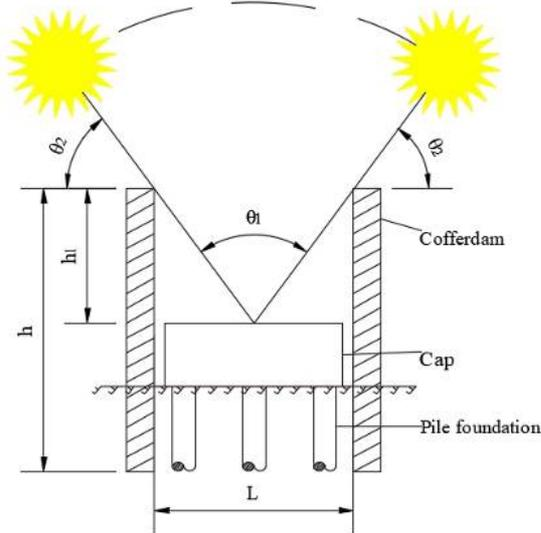
Fig. 2. Calculation diagram for the direct solar angle at the cap center
