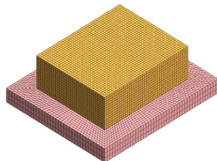
Fig. 6. Finite element model of the massive concrete cap
