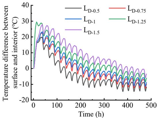
**Fig. 18** Temperature difference time history curve between the inside and the outside of the cap
