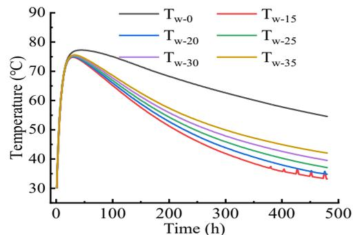
**Fig. 20.** Time history curve of maximum temperature inside the cap
