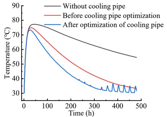
Fig. 24. Maximum transient temperature time history curve of the cap
