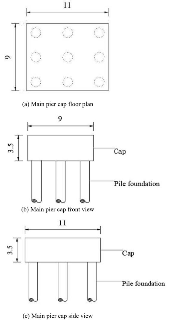
Fig. 5. Dimensional drawing of the cap (unit: m)
