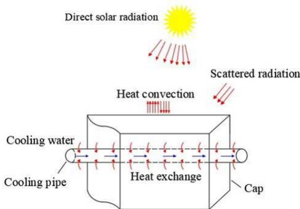
Fig. 1. Heat exchange mechanism of the massive concrete cap
