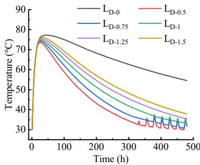
**Fig. 17.** Maximum temperature time history curve inside the cap
