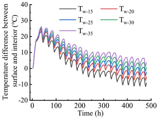
Fig. 21. Temperature difference time history curve between the inside and the outside of the cap
