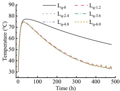
Fig. 22. Time history curve of maximum temperature in the cap
