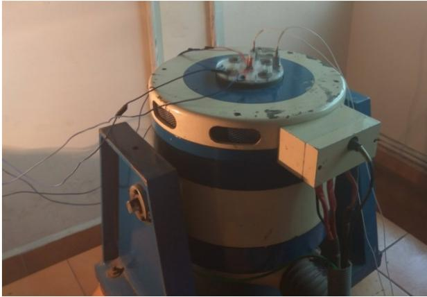
Fig. 5. Electro dynamic shaker with relay mounted
