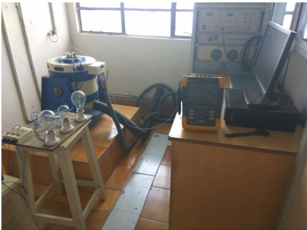
Fig. 6. Experiment setup for Relay Vibration Analysis
