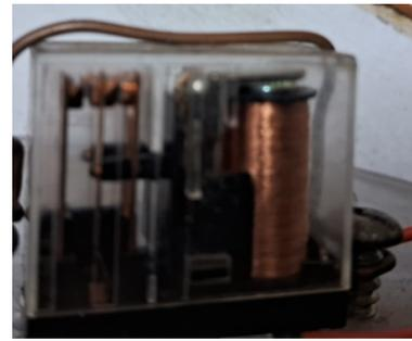
Fig. 1. Electrical Relay
