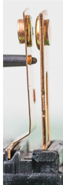
Fig. 2. Electrical Contact
