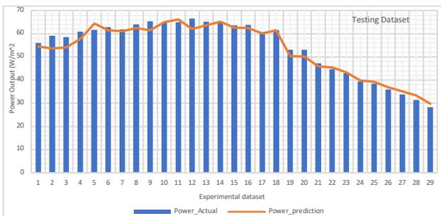
Fig. 8. Comparison of Power generation using the Proposed Hybrid System and the predicted power utilizing the Theory of Experimentation.
