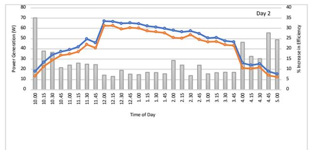
Fig. 5. Indicates the comparison of Power generation using the Proposed Hybrid System and Reference Photovoltaic Panel and the percentage increase in efficiency.
