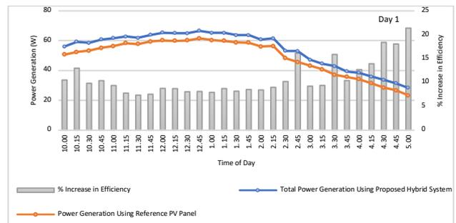
Fig. 4. Comparison of Power generation using the Proposed Hybrid System and Reference Photovoltaic Panel and percentage increase in efficiency.
