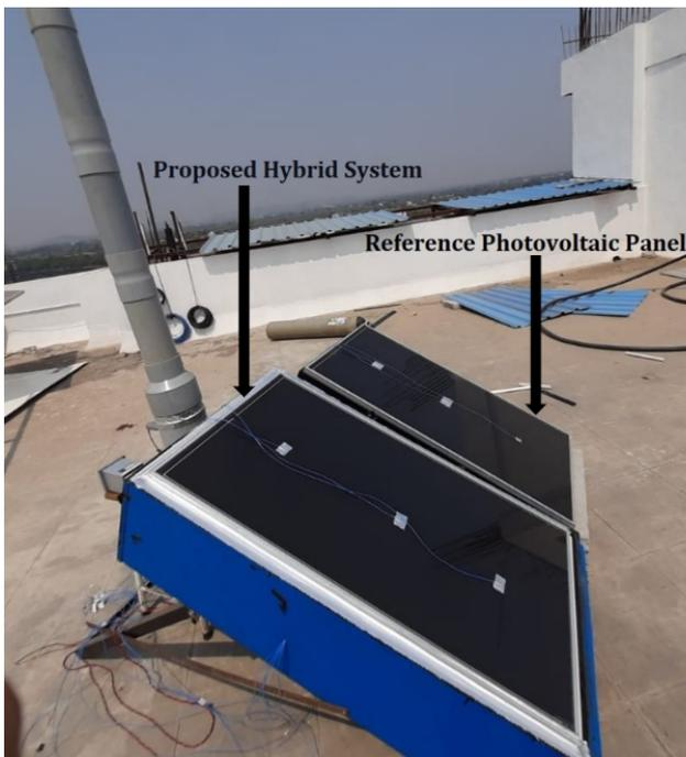
Fig. 2. The actual Image of the Hybrid System & Reference Photovoltaic Panel.
