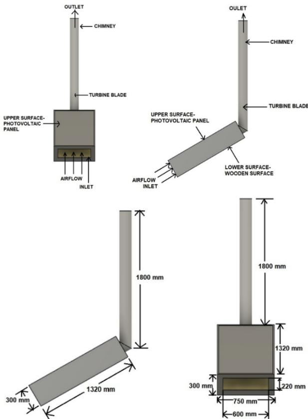
Fig. 1. Indicate the side & front view of the proposed system with Essential parts and dimensions considered in the present work.
