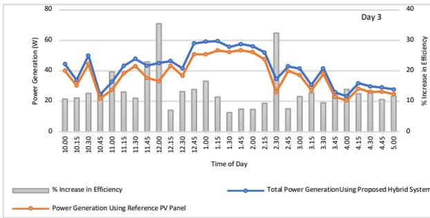
Fig. 6. Indicates the comparison of Power generation using the Proposed Hybrid System and Reference Photovoltaic Panel and a percentage increase in efficiency.
