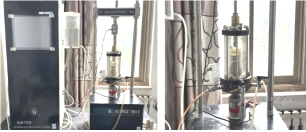
Fig. 2. TSZ-3A automatic strain-controlled triaxial instrument.
