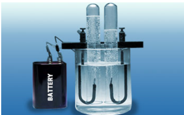
Fig. 1. Electrolysis of water using a battery as an energy source gives H 2 gas at cathode and O 2 gas at anode [8].
