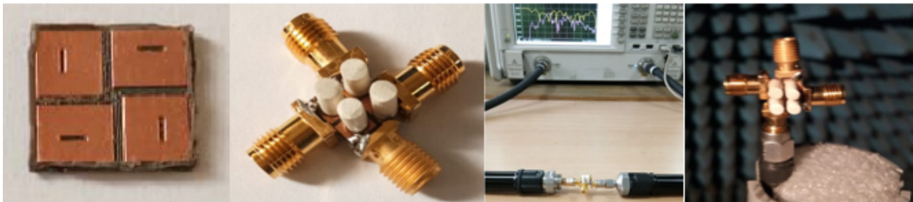
Fig 4. Fabrication of prototype model (a)Top view of a substrate showing slot (b) DRA loaded on slotted patch(c)Model with connectors of VNA (d) R radiation pattern measurement.
