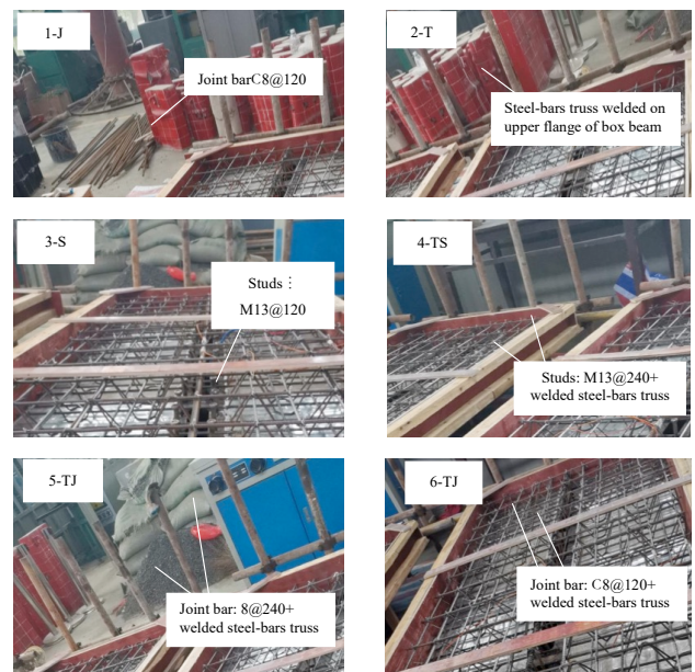
Fig. 3. Layout of shear connectors in each specimen
