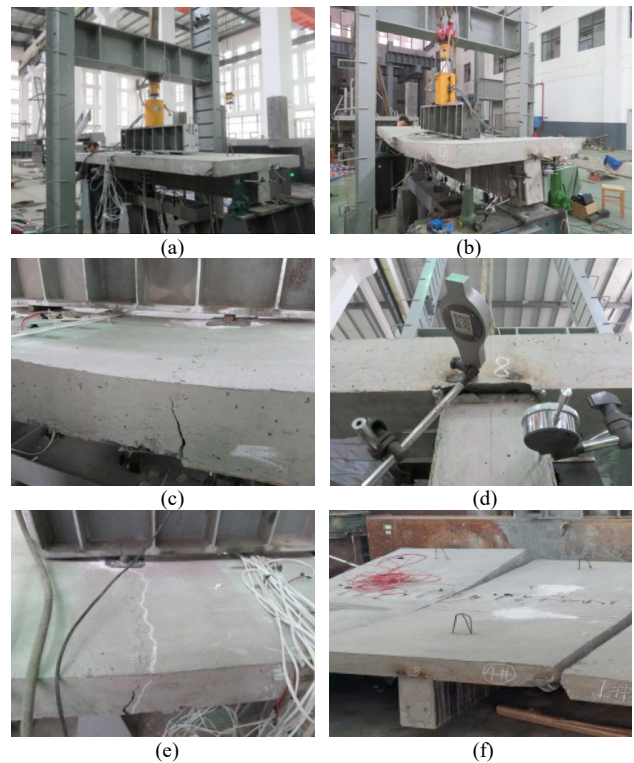
Fig. 10. Failure phenomenon of specimen 4-TS during loading. (a) Before loading. (b) Evident bending of the specimen after loading. (c) Crack of concrete floor slab at loading point. (d) Evident staggered slip at the right end of the specimen. (e) Through crack of the concrete panel at loading point. (f) Final failure mode of the specimen
