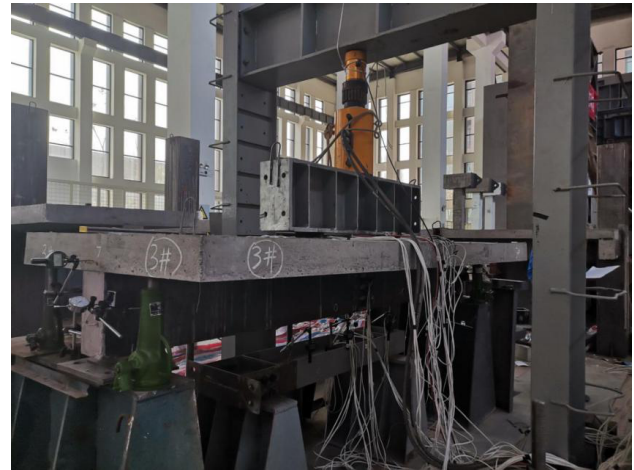
Fig. 5. Actual loading device of composite beam
