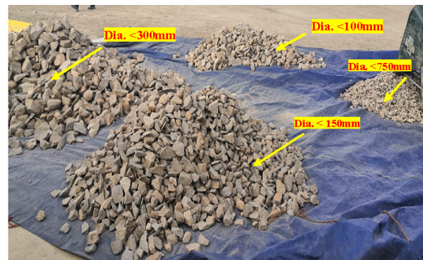
Fig. 2. Jaw-crushed material sieving
