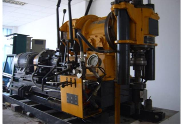
Fig. 5. Test bench of the rock breaking performance of bit
