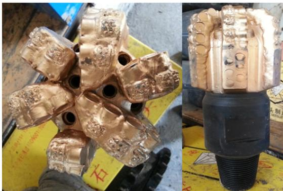
Fig. 2. Physical photo of the SXXXH PDC-DIC hybrid bit
