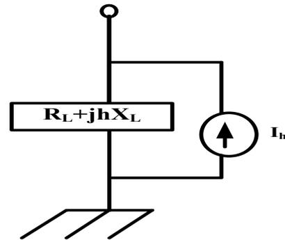
Fig. 5. Representation of the load in a harmonic environment
