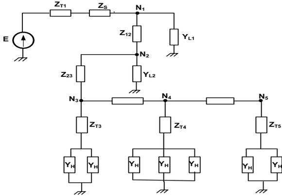
Fig. 3. Circuit representation of distribution system
