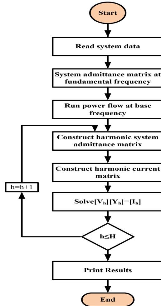
Fig. 1. Flowchart for decoupled the harmonic power flow
