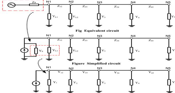
Fig. 4. Circuit reduction of distribution system
