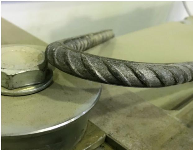
**Fig. 2.** Physical tests of rebar steel, a- Tensile testing curve, b- Bending test.
