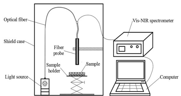
Fig. 1. Sketch of the Vis-NIR detection system
