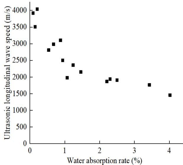
Fig. 8. Longitudinal wave velocity and water absorption rate of stone artifacts from Yue Temple.
