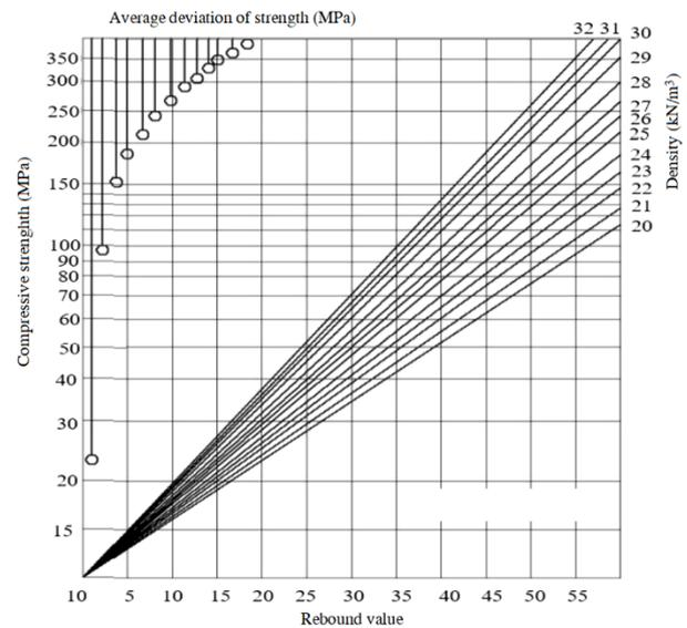
Fig. 1. Rock strength versus rebound value.
