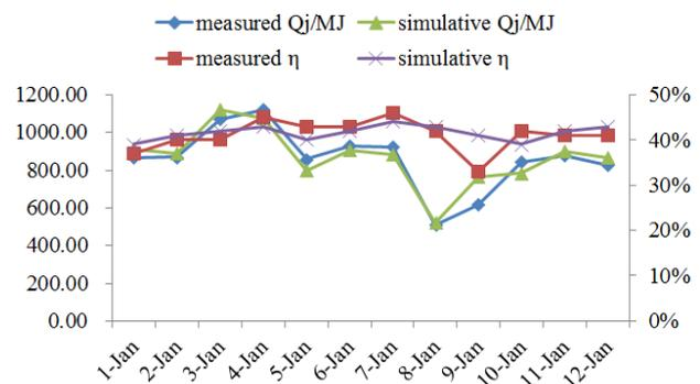
Fig. 4. Comparison between measured values and simulated values of system heat gain and heat collection system efficiency
