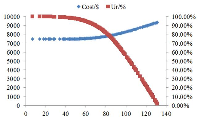
Fig. 6. Annual total cost and solar energy utilization rate of different numbers of household heat-pump water heaters
