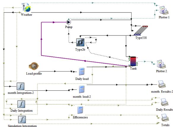
Fig. 2. TRNSYS simulation system diagram
