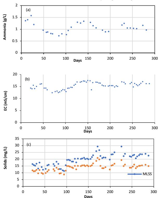
Fig.1. Evolution of (a) ammonia nitrogen, (b) electrical conductivity and (c) suspended solids concentrations of the anaerobic digester effluent during the study period
