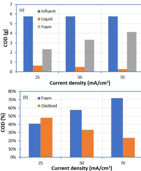
Fig. 3. (a) Mass balance of influent, effluent and foam COD, and (b) percentage of COD transfer to the foam and oxidized, by the applied electrooxidation process at different current densities after 4.5 h processing time.
