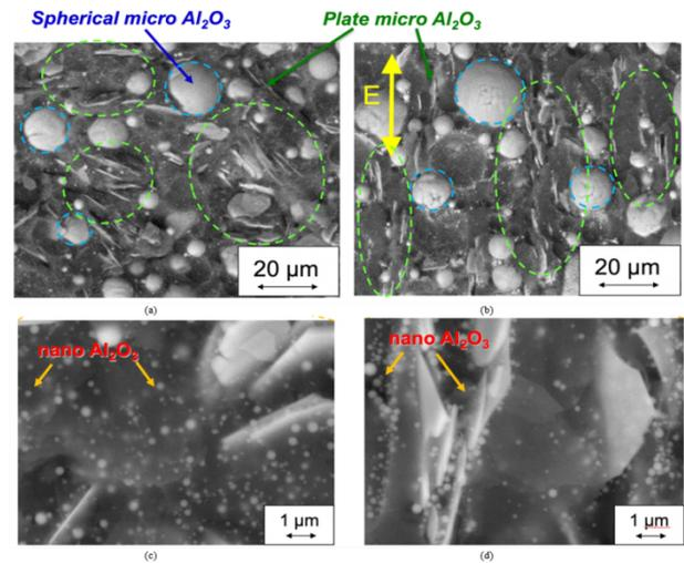
Fig.7. SEM images and enlarged ones of nano and micro  $Al_2O_3$  fillers added epoxy resin  $n+\mu PS$  and  $n+\mu PS-E$  with and without the electric field alignment, respectively. (a)  $n+\mu PS$  (without field; homogeneous dispersion), (b)  $n+\mu PS-E$  (with field; filler alignment), (c) Enlarged SEM of center region of (a) and (d) Enlarged SEM of center region of (b).
