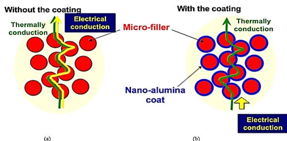
**Fig.11.** Thermal and electrical conduction paths in epoxy matrix containing conductive particles with and without nano-alumina coating. (a) Without nano-alumina coating and (b) with nano-alumina coating.
