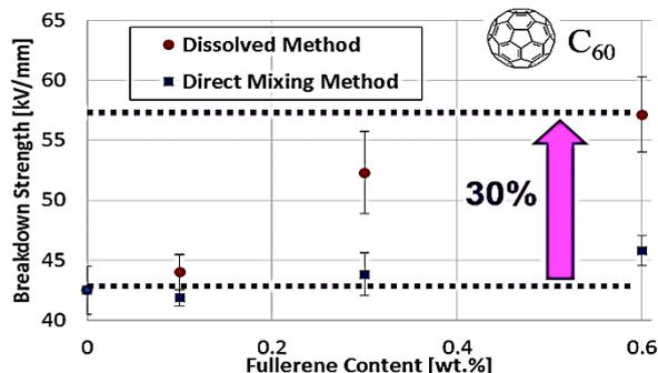
**Fig.12.** Fullerene content dependence on breakdown strength of epoxy composite prepared with the dissolved method and the direct mixing method.
