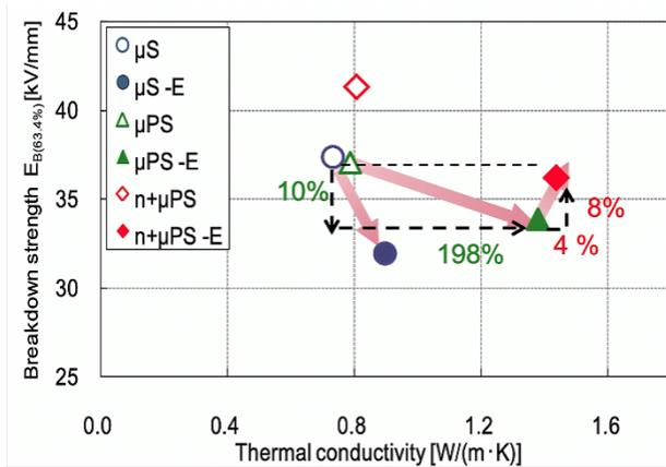
Fig.6. Relation between breakdown strength and thermal conductivity of various type alumina fillers added epoxy resin composites with and without the electric field application E of 2 kV/mm. n stands for nano-sized  $Al_2O_3$  of 1 vol%,  $\mu S$  : micro-sized spherical  $Al_2O_3$  of 35 vol%,  $\mu PS$  : micro-sized plate-like and spherical  $Al_2O_3$  of 7 and 28 vol%, respectively.
