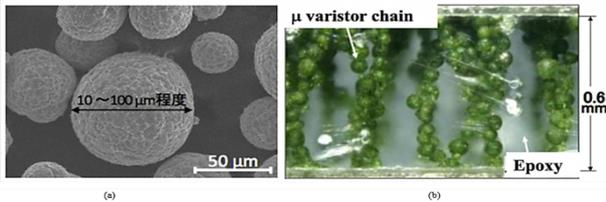
Fig.8. Microvaristor particles and epoxy composite varistor with field application. (a) Microvaristor particles and (b) Composite varistor.
