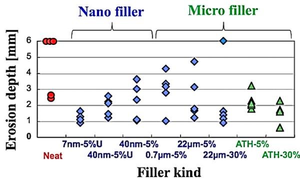
**Fig. 1.** Average erosion depth for each specimen after the inclined plane test. U and ATH stand for nanocomposites prepared using an ultrasonic homogenizer and composites mixed with micro-sized acid tri-hydrate filler.
