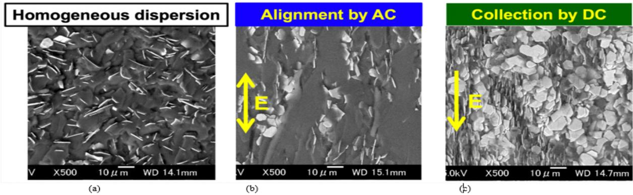
Fig.5. SEM image of plate-like alumina filler orientation by AC and DC electric field E application during curing process of epoxy resin. (a) 10 vol%,  $\kappa = 0.34$  W/m K (b) 10 vol%,  $\kappa = 0.73$  W/m K (c) 20 vol% (locally 40 vol%),  $\kappa = 9.87$  W/m K.
