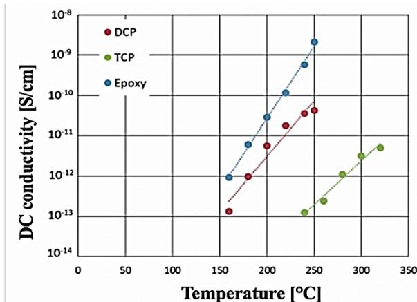
**Fig. 3.** Temperature dependence of DC conductivity of P-DCP and P-TCP as compared with that of epoxy resin.
