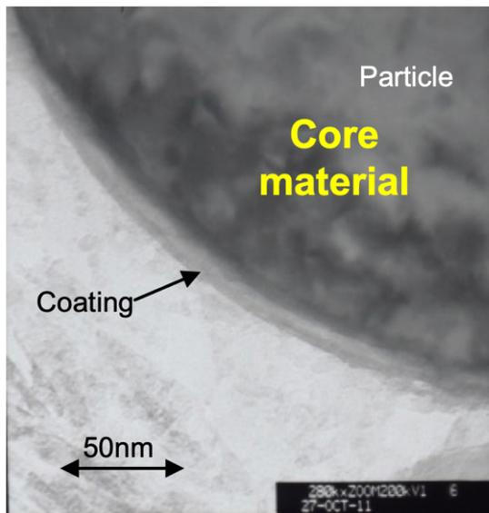
Fig. 10. TEM image of nano-alumina coated spherical aluminum.
