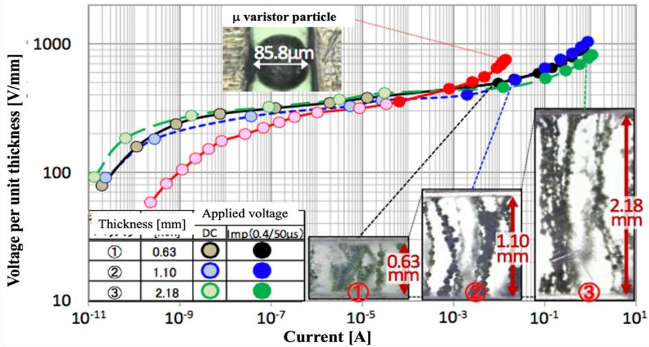
Fig. 9. Voltage-current characteristics of composite varistor with different thicknesses.
