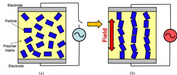
**Fig. 4.** Principle of electric field orientation of filler in matrix polymer. Coulomb force due to polarization charge forms filler chain structure. (a) Before electric field application and (b) Electric field application during cure process.
