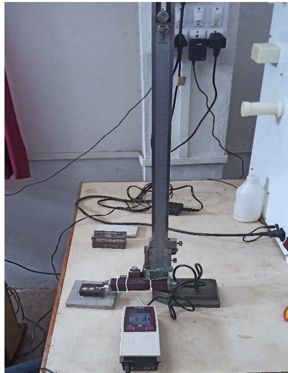
Fig. 1. Surface roughness test setup
