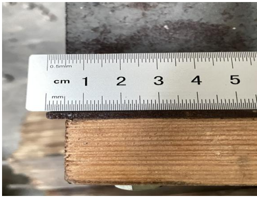
(c) Slip of lower flange relative to steel web
