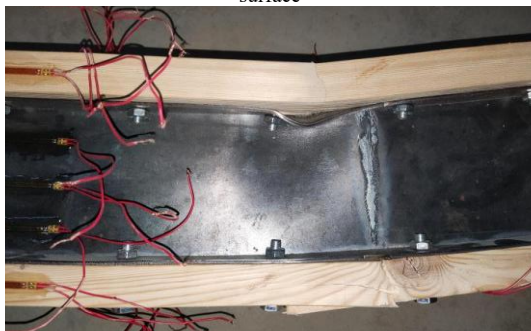
(l) Buckling of beam L3 steel web upper exterior
