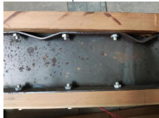
(f) Buckling of beam L1 steel web upper exterior
