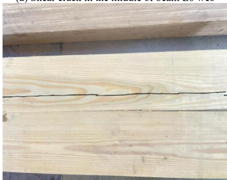
(b) Local longitudinal crack on beam L0 top surface
