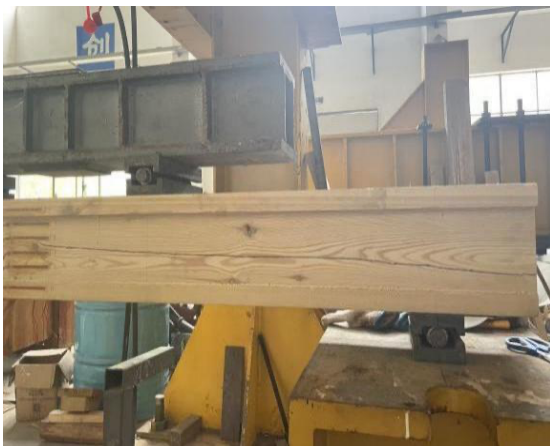
(a) Shear crack in the middle of beam L0 web
