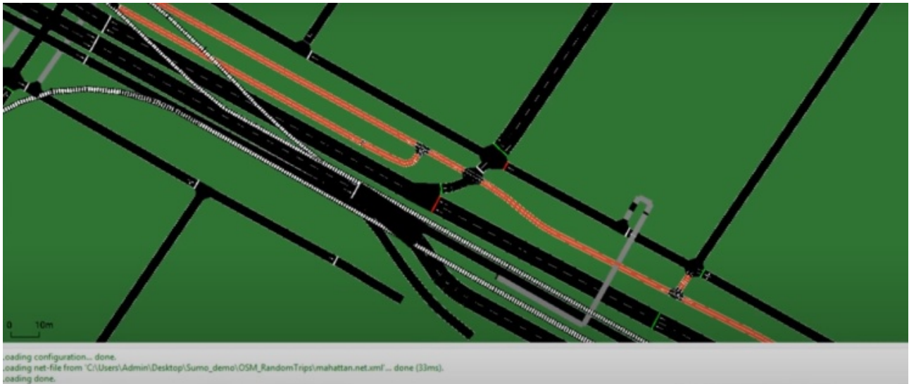
Fig. 6. Network file running in Simulation for Urban Mobility (SUMO)
