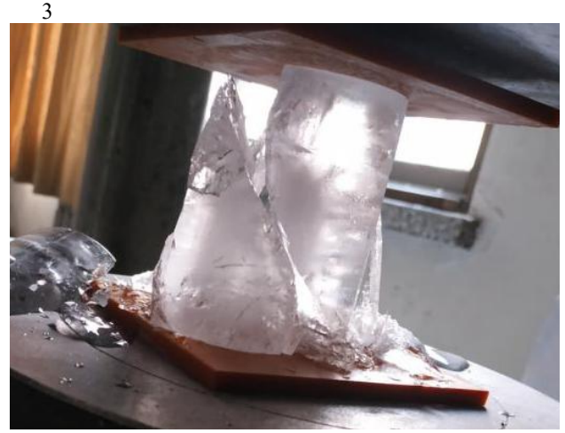
Fig. 7. Damage pattern of icicles.
