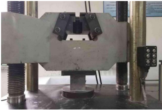
(a) The compression test of an ALWSSC specimen
