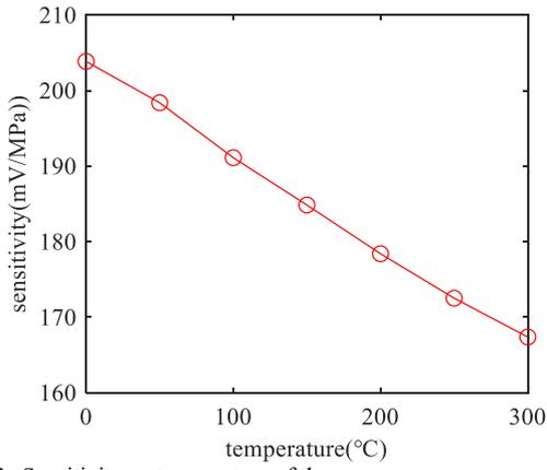
Fig. 8. Sensitivity vs temperature of the sensor
