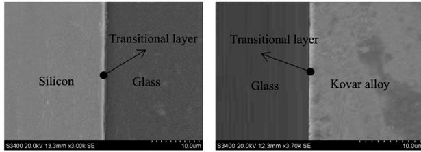
Fig. 7. Bonding interface between silicon and glass, glass and kovar alloy
