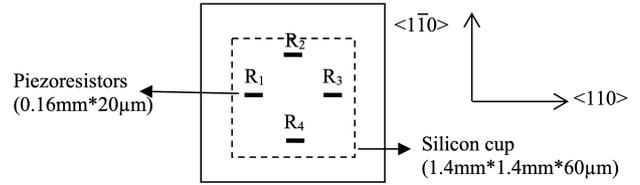
Fig. 1. Piezoresistors arrangement on the square diaphragm [25]3.3 Smart-Cut SOI
