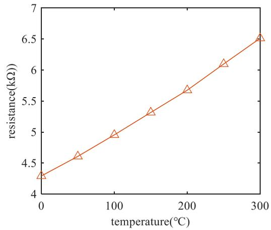
Fig. 11. Resistance vs temperature of the sensor
