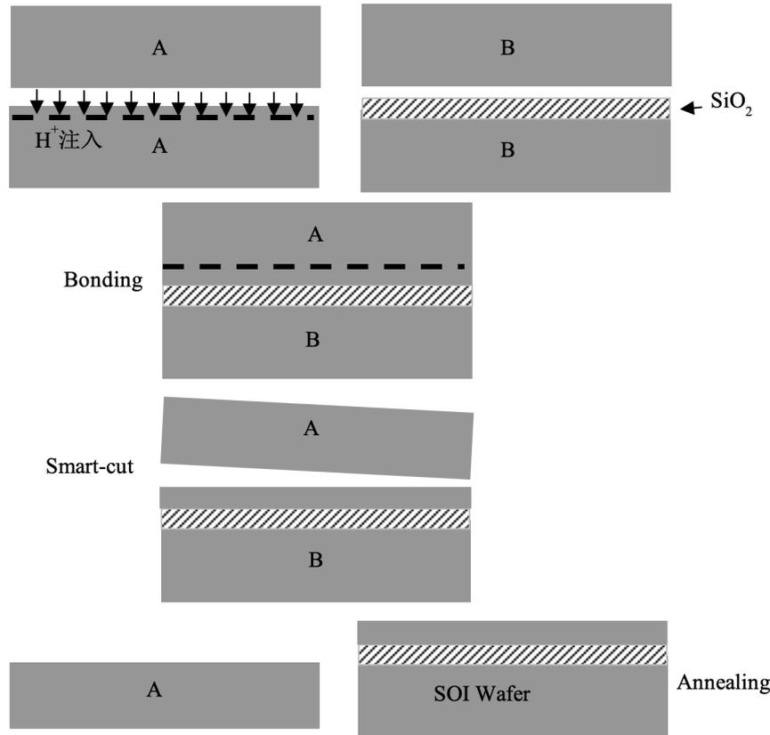
Fig. 2. Smart-cut process for SOI wafer
