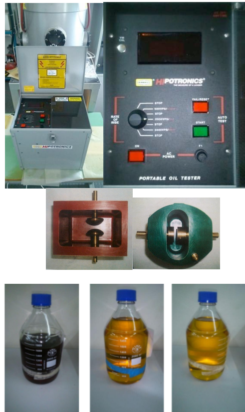
Fig. 1. Typical Foster test cell experimental device (up -left), front picture (up - middle), testing cells with adjustable gap (middle – left) Bruce profile on uppers and flat on bottom). Rate selections were 500Vps, 2000Vps and 3000Vps. The characteristics of the three oils (at the bottom, N1A, N2B, N3A) are described in the text. [Shots where taken from the lab]
