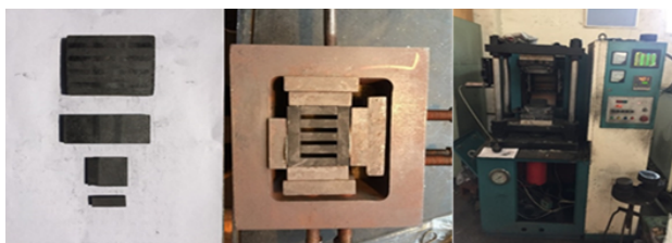
(a) Graphite mold, (b) matrix fixture, (c) RJY2000A sintering machine Fig. 3. Hot-pressing sintering mold and furnace
