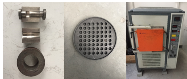
(a) Matrix steel mold, (b) Graphite mold, (c) Vacuum sintering furnace Fig. 4. Cold-pressing calcination model and sintering furnace
