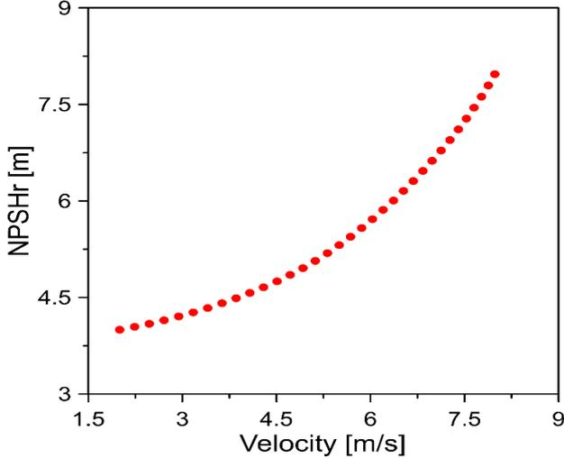
Fig. 8. Net positive suction head required.
