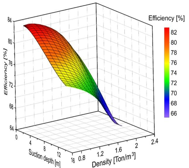
Fig.10. Pump efficiency with respect to density and suction depth parameters.
