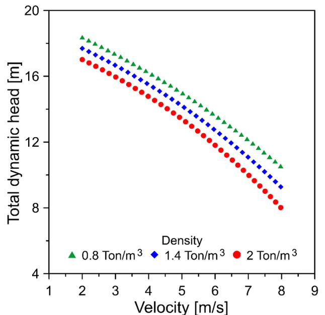
Fig. 7. Effect of slurry density on the total dynamic head.
