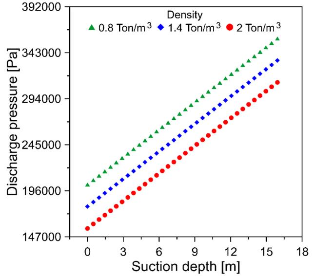
Fig. 4. Relationship between the discharge pressure and suction depth.
