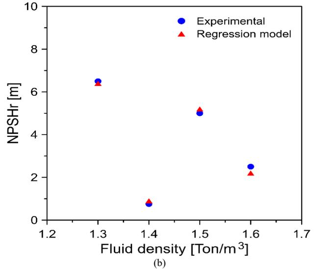
Fig. 9. Comparison between the NPSHr obtained experimentally and using the regression model according to (a) Suction depth and (b) fluid density.
