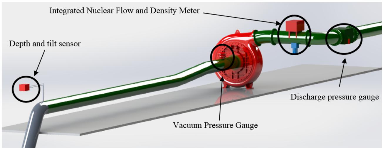
**Fig. 2.** Experimental assembly and instruments used
