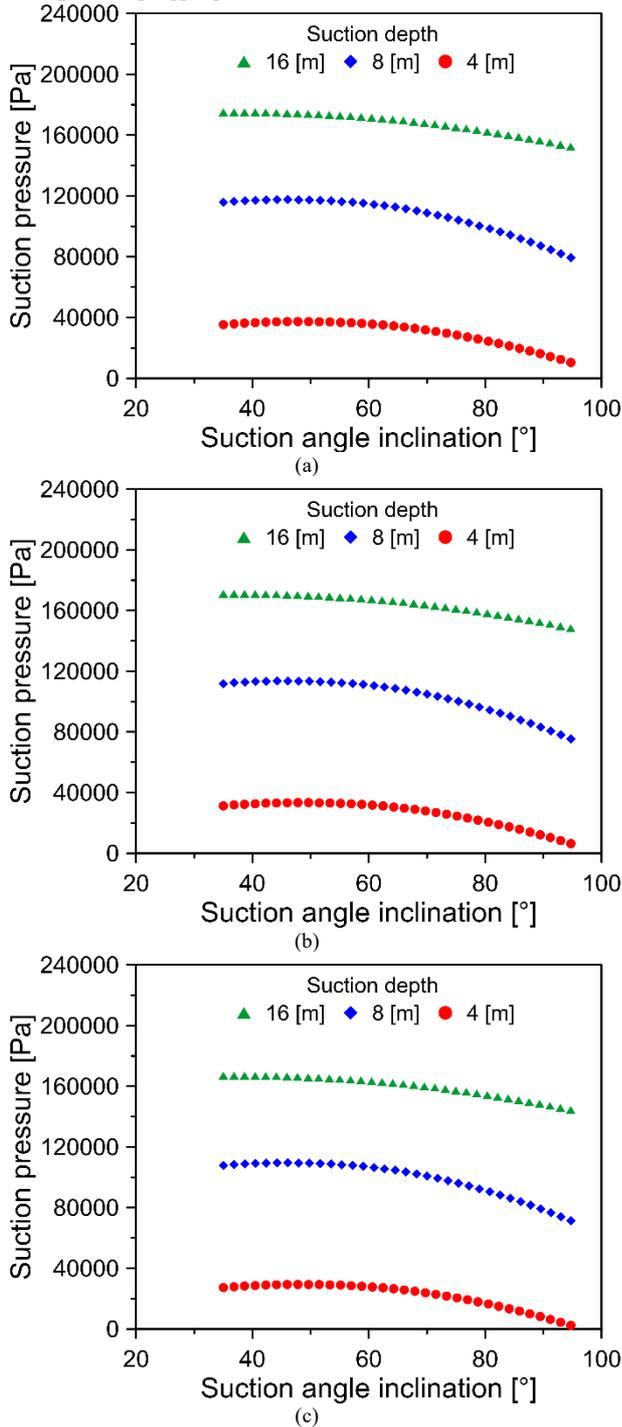
Fig. 5. Relationship between the suction pressure and the inclination of the suction angle for (a) 0.8 Ton/m<sup>3</sup>, (b) 1.4 Ton/m<sup>3</sup> and (c) 2 Ton/m<sup>3</sup>.
