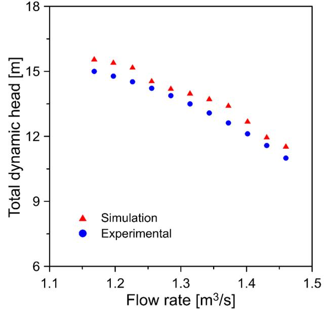
**Fig. 4.** Characteristic curve of the pump obtained experimentally and numerically.
