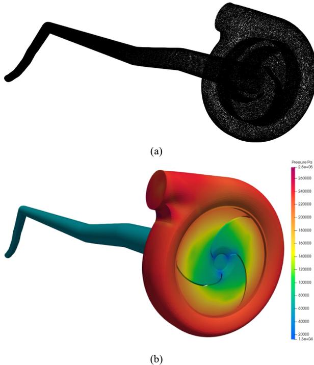
**Fig. 3.** CFD analysis a) Mesh used in study b) pressure profile inside the pump
