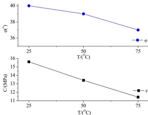
Fig. 14. Relation between cohesion, internal friction angle and temperature
