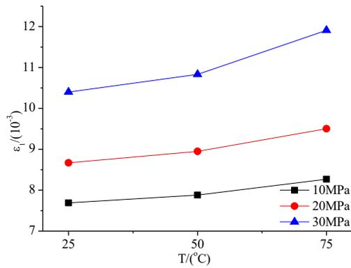
Fig. 12. Axial peak strain and temperature relation at different confining pressures
