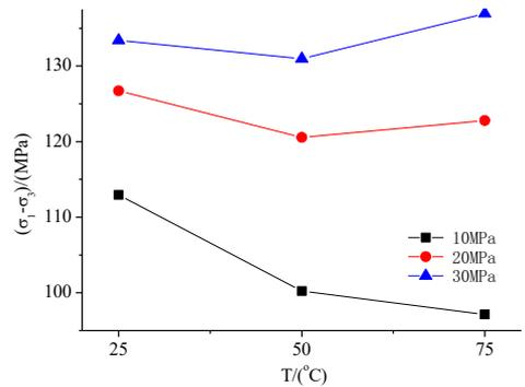
**Fig. 8.** Axial failure load and temperature relation at different confining pressures
