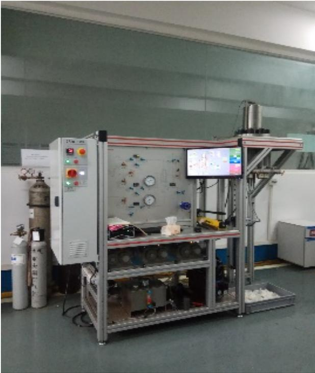
Fig. 1. Rock Multi-field Coupling Triaxial Instrument
