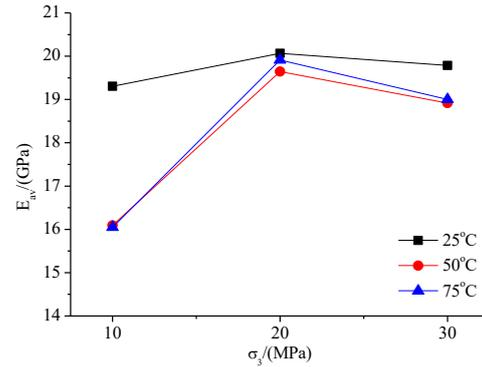
Fig. 10. Average modulus and confining pressure relation at different temperatures
