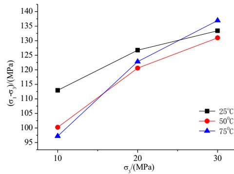
**Fig. 7.** Axial failure load and confining pressure relation at different temperatures
