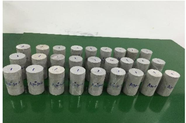
Fig. 3. Sandstone Test Pieces
