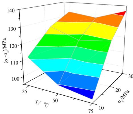
Fig. 9. 3D stress diagram showing axial failure load, confining pressure, and temperature
