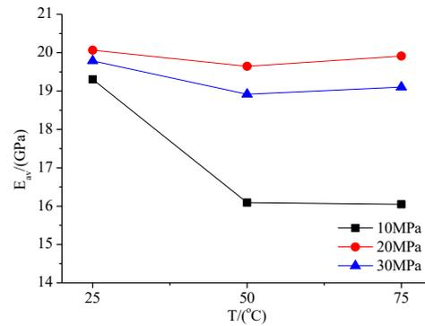
Fig. 11. Average modulus and temperature relation at different confining pressures
