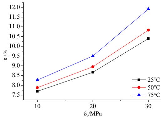
Fig. 13. Axial peak strain and confining pressure at different temperatures
