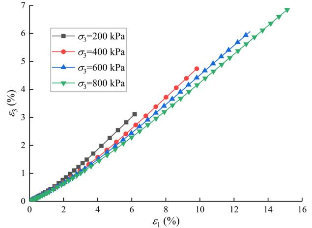
**Fig. 14.**  $\varepsilon_1 \sim \varepsilon_3$  relation curves of the samples under different confining pressures
