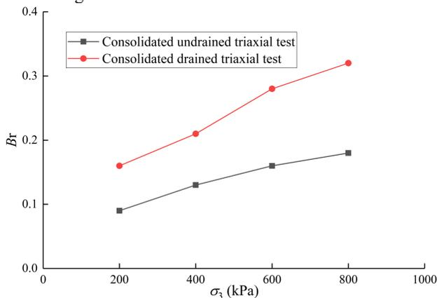
Fig. 11. Relation curves between grain breakage index and confining pressure
