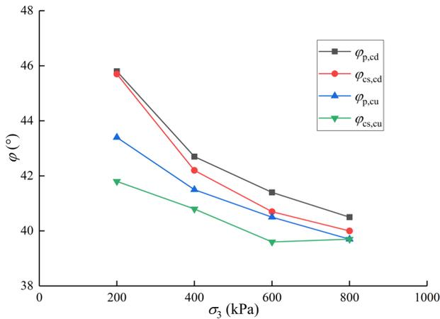
Fig. 10 Change curves of peak friction angle and critical friction angle with confining pressure
