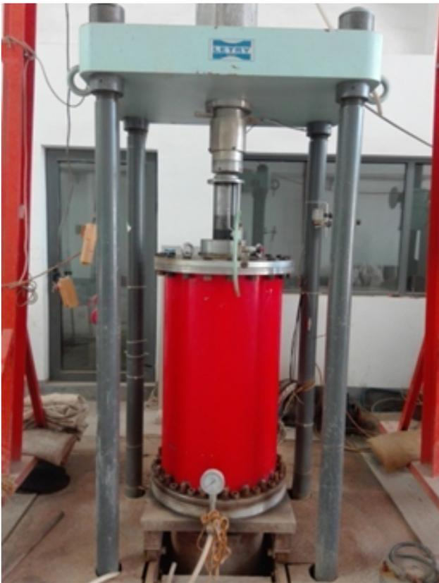
Fig. 1. Large static triaxial apparatus
