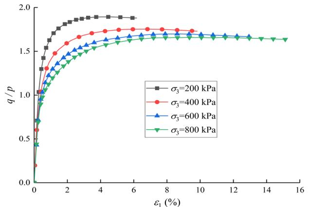
Fig. 5 Relation curves between generalized shear stress ratio-axial strain of the sample under drained condition
