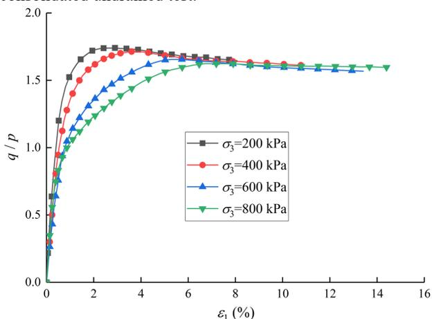
Fig. 6. Relation curves of shear stress ratio-axial strain of sample under undrained condition
