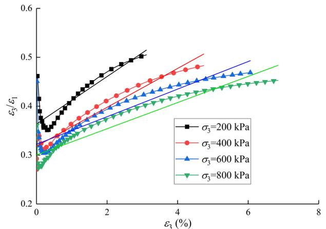
**Fig. 15.**  $\varepsilon_3 / \varepsilon_1 \sim \varepsilon_1$  relation curves of the samples under different confining pressures
