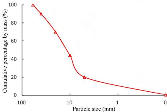
Fig. 2. Grading curve of embankment filler used in the test
