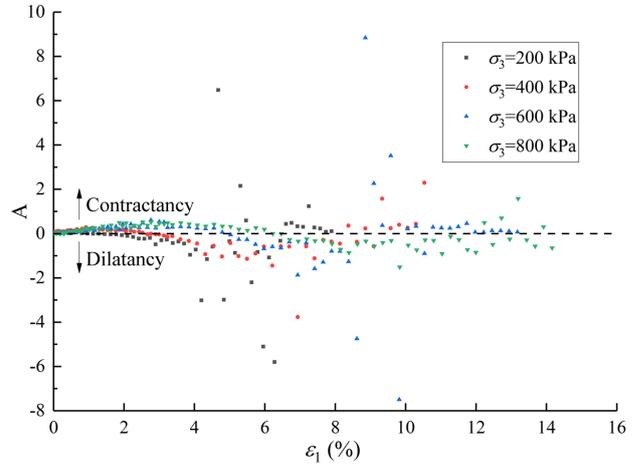
Fig. 9. Relationship between pore water pressure coefficient and axial strain
