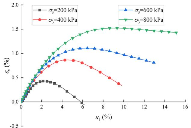
Fig. 7. Relation curves of volumetric strain-axial strain of the sample under drained condition
