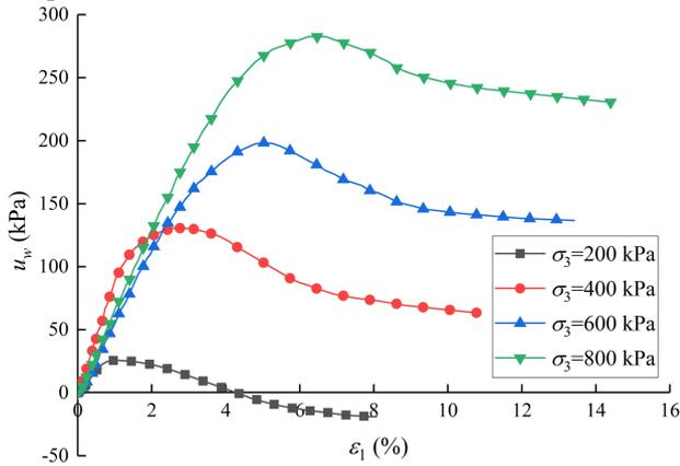
Fig. 8. Relation curves of pore water pressure-axial strain of sample under undrained condition
