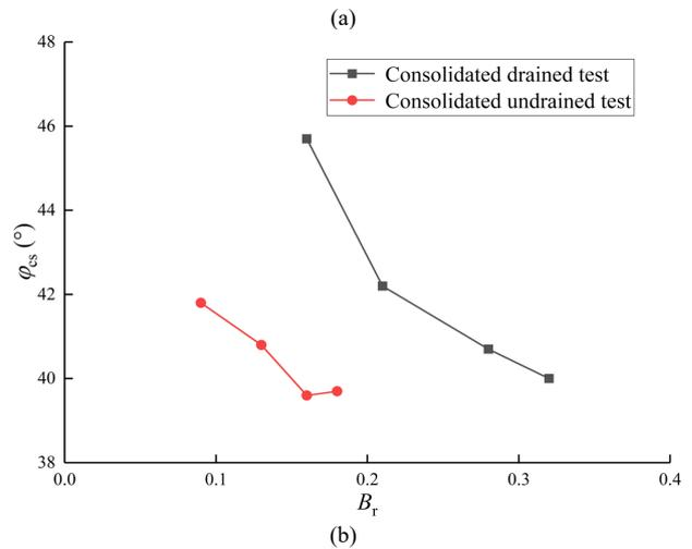
Fig. 12. Change curves of the peak and critical friction angles with grain breakage index
