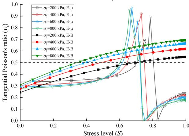
**Fig. 13.** Relation curves of the Poisson’s ratio and stress level of the sample obtained through  $E \sim \mu$  and  $E \sim B$  models under different confining pressures
